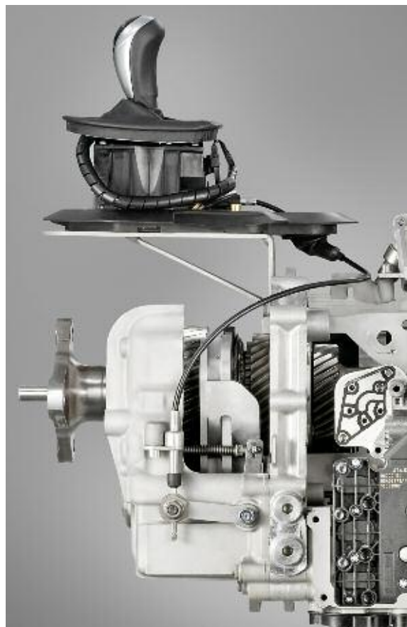
M DCT parking lock lever, (cut away view from rear right of transmission)
