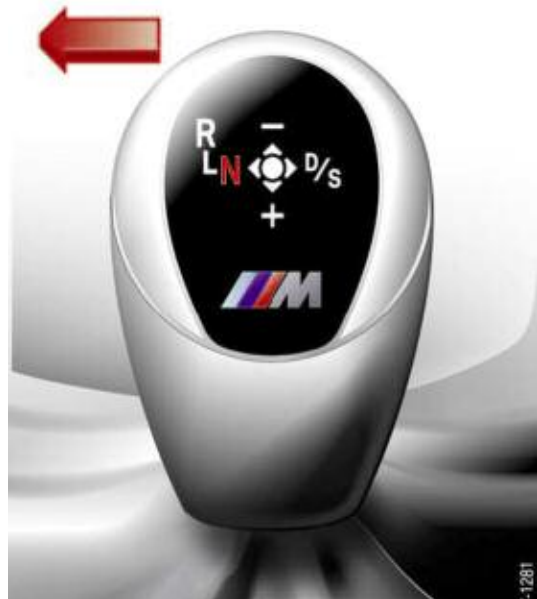
The M GWS one-touch function is pushed to the left to shift into neutral.
