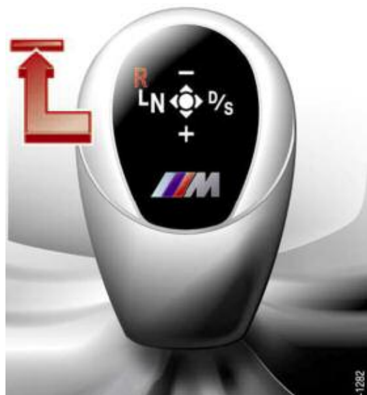
M GWS Reverse gear position
