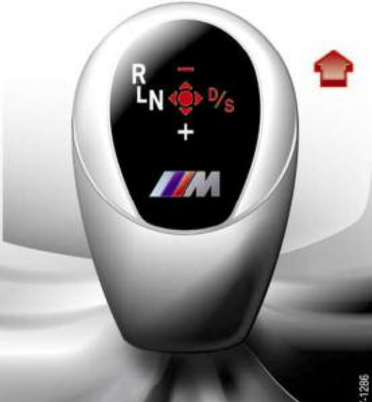
M GWS in sequential mode, downshifting.
