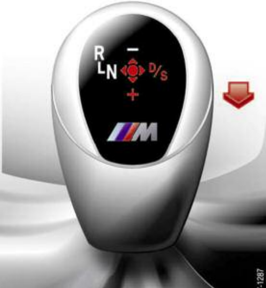
M GWS in sequential mode, upshifting.
