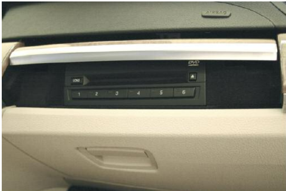
Single-slot DVD changer is located behind dashboard trim panel above the glove compartment
