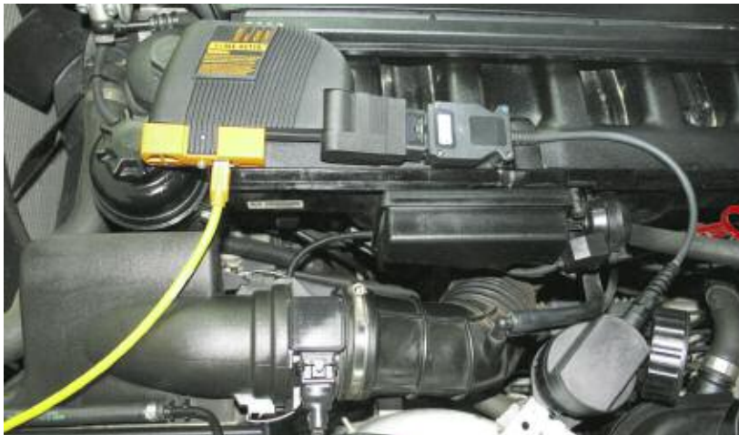
Vehicle access for I-bus/K-bus vehicles
