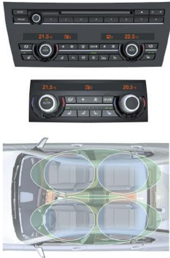
Control panel for IHKA with FKA rear climate control with IHKA 4 zone.
