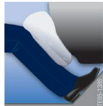
Knee airbag in operation
