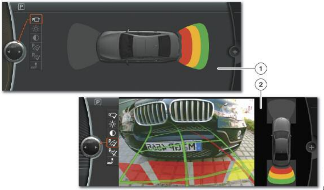
Distance warning PDC display and option to select rear view camera image with PDC
