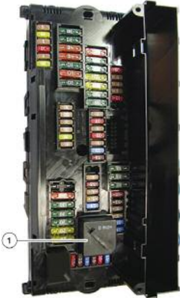
Front view of the front fuse carrier in the F01//F02
