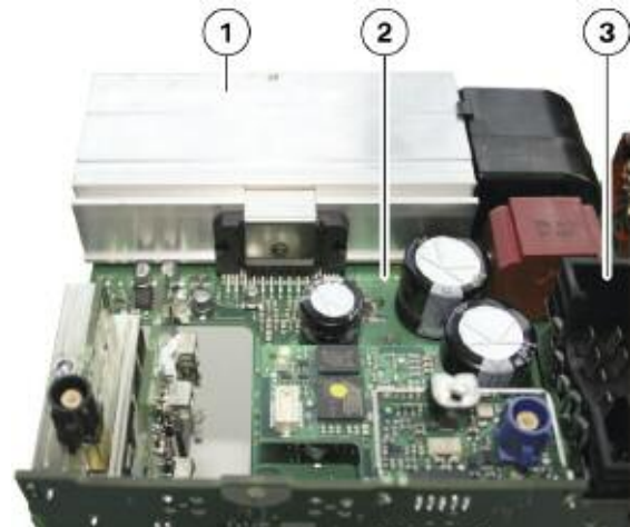
CIC Main Board and Heat Sink Location
