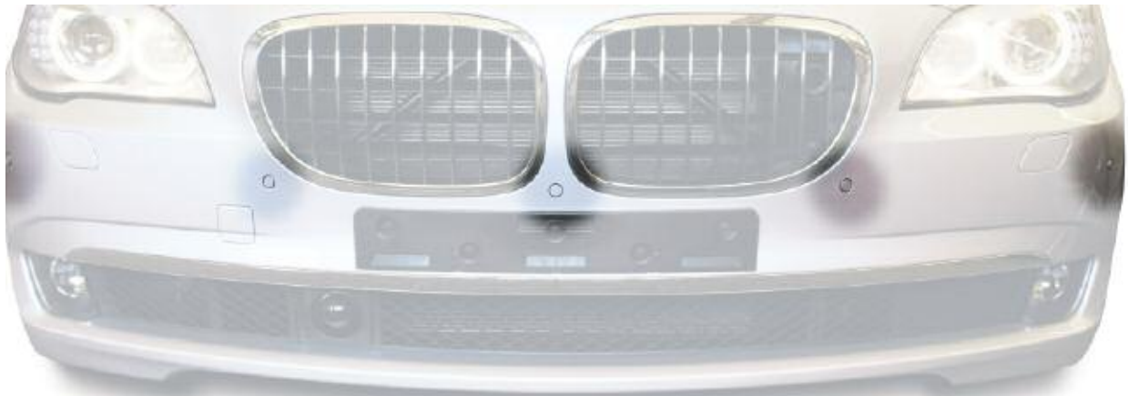
F01/F02 front bumper with five Park Distance Control ultrasonic sensors
