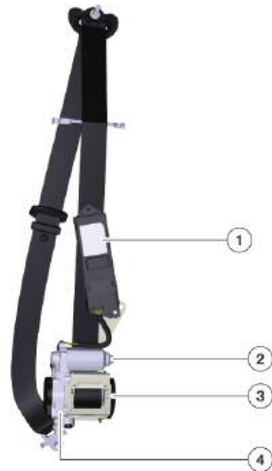
Seat belt with electric motor driven reel
