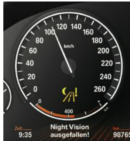
Display indicating defective system
