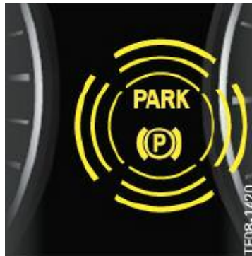
Indication of parking-brake installation mode
