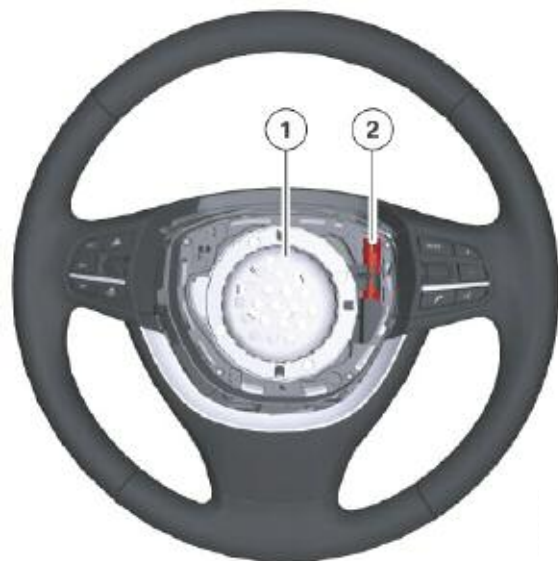
Driver airbag without airbag
