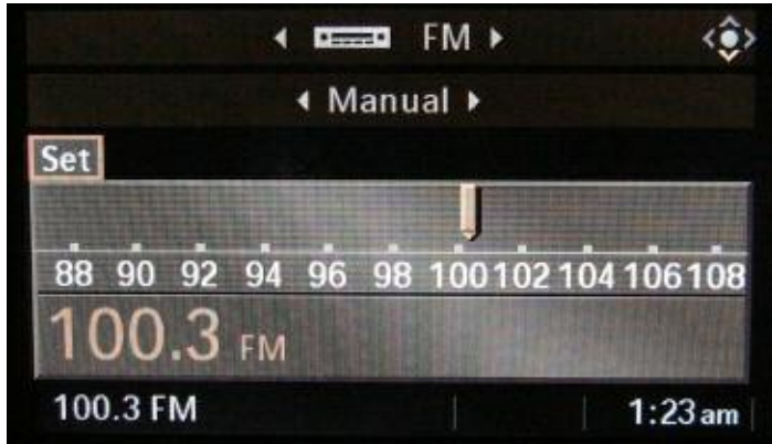
Manual station search in a CCC system
