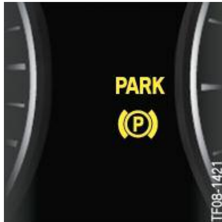
Indication of “parking brake emergency release/fault”
