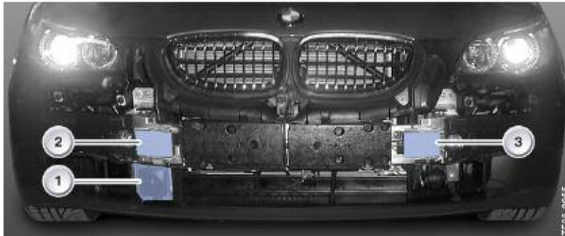
Radar sensors for ACC Stop & Go, Front view
