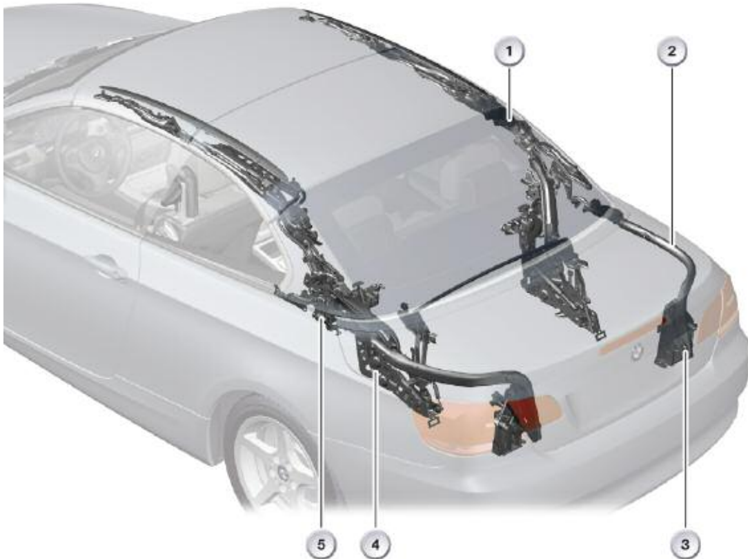
Mechanism of the E93 retractable hardtop
