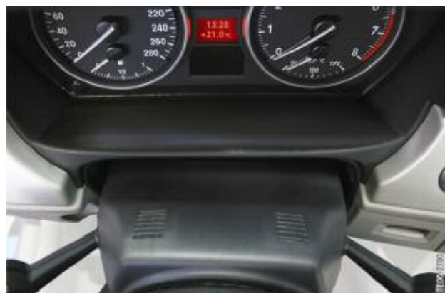
Location of microphones for phone and voice input
