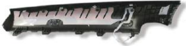
AM and FM1 antenna in LH trim panel
