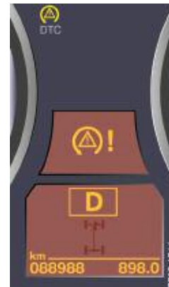
Display in the event of a DPC system failure
