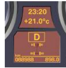
Dynamic Performance Control display with small symbol and odometer reading (displayed upon engine startup)
