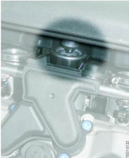
Oil separator connection point to the intake manifold
