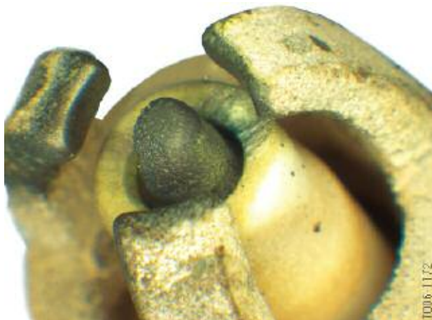
The spark plug above shows erosion of the electrode on one side which could be an indication of fuel spray "diversion".
