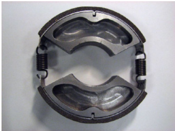
Clutch Material with Springs and Weights
