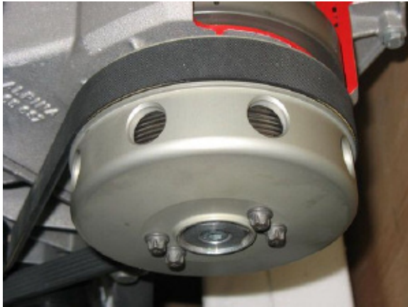
Bell Housing/Pulley Installed
