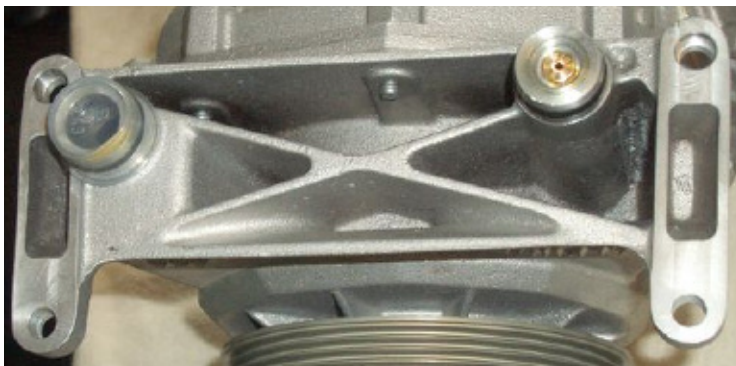
Supercharger - Oil Restricting Orifice (Right)
