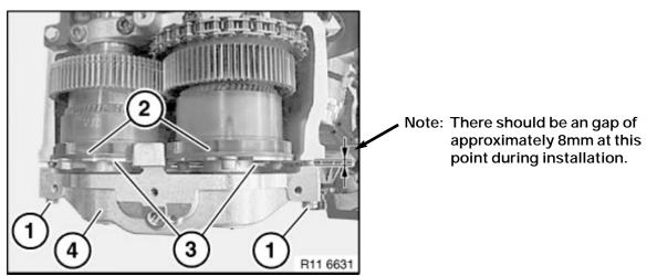
Install VANOS adjusting unit (with gasket). Position the adjustment unit using the outer bolts (1), but <u>do not tighten</u> bolts. Ensure that the VANOS gears (2) are fully extended. Align thrust plates (3) and make sure that the thrust plates are flush with the VANOS gears. Install the (exposed) hex (Allen) bolts, tighten and then loosen 90 degrees.
