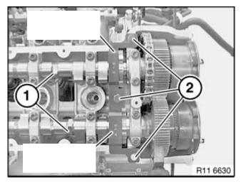
Install special tools as shown above, write correct tool numbers in spaces provided. Be sure to fully tighten all bolts (see 2 above).
