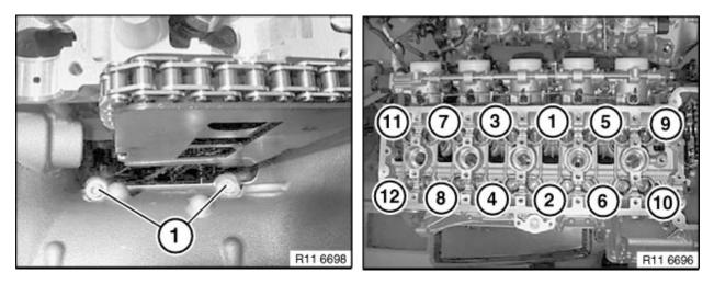
Remove cylinder head and inspect piston installation for reference. Note coolant and oil passages.
