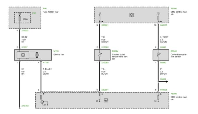
The cooling fan is controlled by the ECM through an output stage which receives a PWM signal. The ECM varies the PWM signal based on the following factors:
