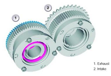
The gear mechanism is driven by the drive gearwheel that interacts with the helical gearing on the inner sleeve. The threaded connections for the gearing connects the inner sleeve to the outer sleeve. With (wide) helical gearing, the inner sleeve acts on the bearing assembly for the drive gearwheel that is firmly secured to the camshaft with the central bolt.
