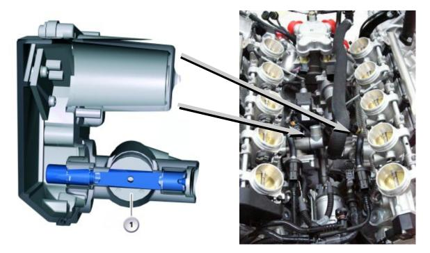
The engine control module determines the current actual load signal from the throttle valve sensors (DKG) and feedback signals from the LLS actuators in order the check the setting of the throttle valves. The plausibility of the load signal is checked against the signals of the two hot-film air mass meters.
