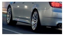
The rear bumper of the vehicle does not only make the vehicle appear more sporty but includes an air diffuser to better improve the aerodynamics of the vehicle.
