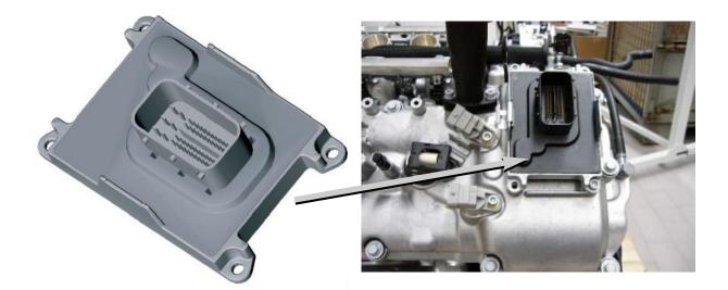
In addition to ignition coil control, the ionic current control unit is used to measure ionic current during the combustion period (after ignition). These measurements are used by the engine management to monitor knock as well as misfiring.
