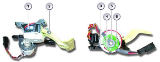
Actuators of the Active Backrest Width Adjustment with Sensors
