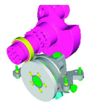
The high pressure pump receives it oil supply from the bedplate. An 80 micron fine filter is installed in the transition hole from the bedplate to the high pressure pump. This filter has the sole purpose of holding back any impurities that may accumulate during series production and is not replaced during vehicle operation.
