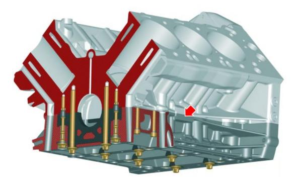
The bedplate is secured to the upper section of the crankcase with the main bearing bolts. The positions are fixed with fitted sleeves. Strict adherence to the bolt tightening procedure is necessary to prevent engine failure.
