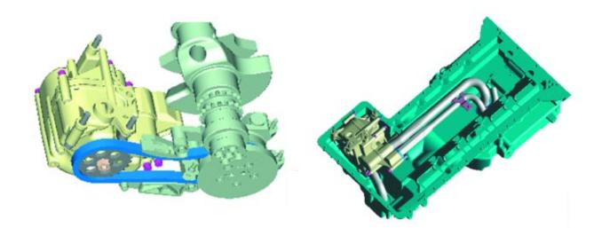
The other pump is a slide-valve design which has a variable displacement capability. The slide valve pump takes the oil from the rear sump and conveys it to the oil filter at a variable pressure of up to 5 bar.
