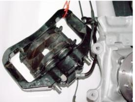
**Dual Piston Front Brake Caliper**
