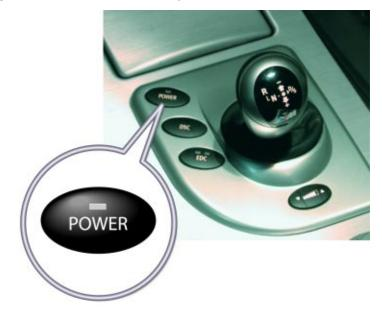
The DME receives the ground input from the switch. The SZM is responsible for the illumination of the "On" LED. Switch illumination is provided by the KL58g circuit.
