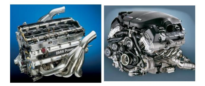
The engine block and cylinder heads are constructed of aluminum alloy and are designed to withstand the demands and stresses of an F1 race. The titanium connecting rods are just one example of components which allow the P84/5 to reach engine speeds of more than 19,000 RPM.
