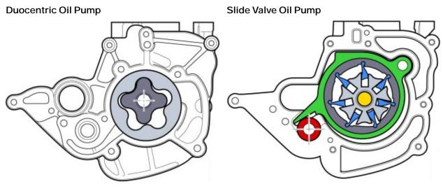
The pump outlet is determined by the eccentricity of the pendulum-type slide valve. No oil is delivered when the pump runs centrally with respect to the rotor as all pump chambers are the same size.
