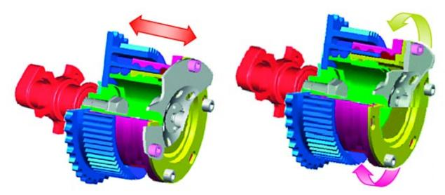
Intake gear mechanism adjustment direction
