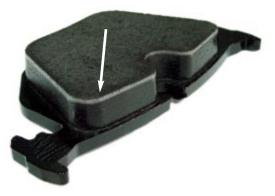
Brake pads are made by gluing the friction material to a backing plate (metal). These are then baked in an oven to allow the glue to cure. While the brakes are heated, gasses are released and travel through the brake pads to the surface. This can be seen on any new brake pads as a lighter upper section of the brake pad (see picture to the left).
