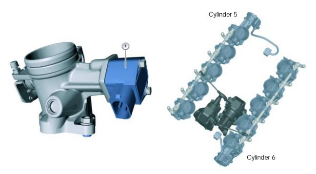
One throttle valve position sensor is located on the throttle housing for cylinder 5 (bank I) and the other is located on the throttle housing for cylinder 6 (bank II). Each sensor contains 2 feedback hall sensors to detect throttle plate position.
