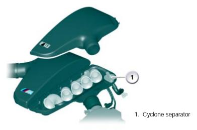
Cyclone separators are installed in the intake air plenums in the area of the fifth and tenth cylinder. The oil from the oil separators and the condensate from the manifolds merge in two channels in the crankcase behind the tenth cylinder and routed into the oil sump.
