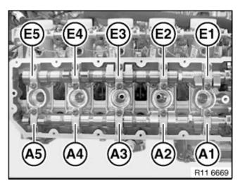
Depress camshafts with special tool and secure bearing caps. Do not tighten the camshaft bearing caps to full specification on the trainer engine.
