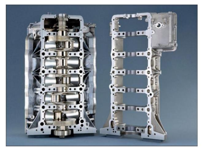
The 10 cylinder crankcase uses the familiar Alusil construction which is split at the crankshaft centerline. The bedplate is machined together with the crankcase and is mounted to the upper section of the crankcase when the engine is assembled. This design contributes to improved torsional stiffness. Better engine acoustics (NVH) are also attributed to the improved stiffness.
