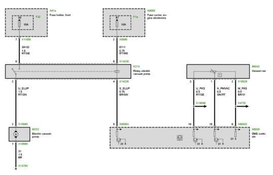
A test module is provided in DIS for the electric vacuum pump. The differential pressure sensor on the brake booster is used for the purpose of monitoring the pump. The plausibility is checked by the pressure difference between the vacuum and ambient pressure calculated internally in the ECM. It is evaluated and, in the case of fault, shown in the instrument cluster and displayed as a CC message (check control).
