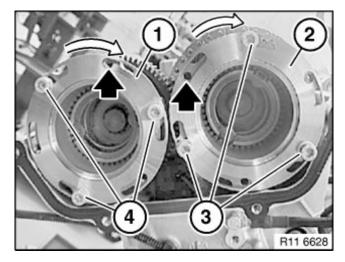
Loosen bolts (3 and 4) but do not remove. Rotate inner sleeve of VANOS gear to the left most stop (refer to graphic above - 1 and 2). Re-tighten bolts (3 and 4) to approximately 5 Nm.
