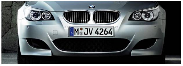
In conjunction with sealing the engine compartment, the front bumper reduces lift on the M5's front axle by 50% in comparison to the standard car.
