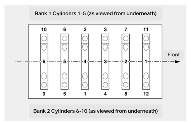
Proceed and install all, M11 main bearing cap bolts. And tighten in sequence (on the trainer engine only tighten to 30Nm).
