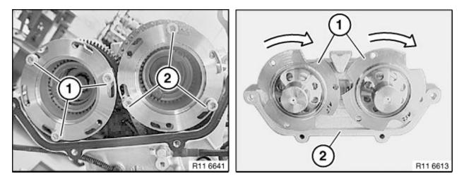
Loosen bolts (see above left picture1 and 2) 90 degrees. Before installing VANOS adjusting unit, ensure that the thrust plates (see above right - 1) are fully retracted and rotate freely without binding.
