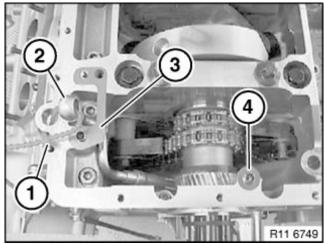
Re-install VANOS pump, note installation position of the shims (3 and 4 above).
