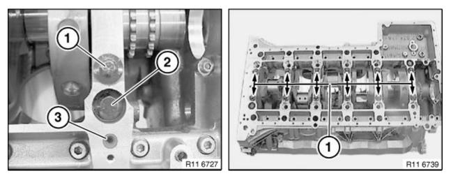
First remove all M8 fit bolts (#2 - above left) completely from engine. Next, remove the M11 main cap bolts (#1- above right). Then proceed by removing the remainder of the hex (allen) bolts.
