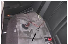
Mechanical Release for Trunk
