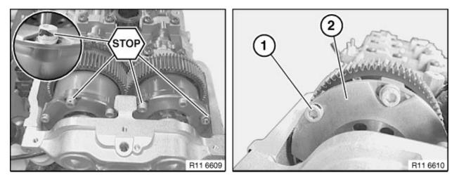
Remove 6 bolts (reference #1 on graphic) on each VANOS adjusting unit, rotate engine to access all bolts on both banks. Proceed with removal of both VANOS adjusting units as per repair instructions.
