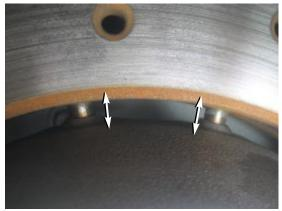
**Detail of Rotor Attachment Pins**
