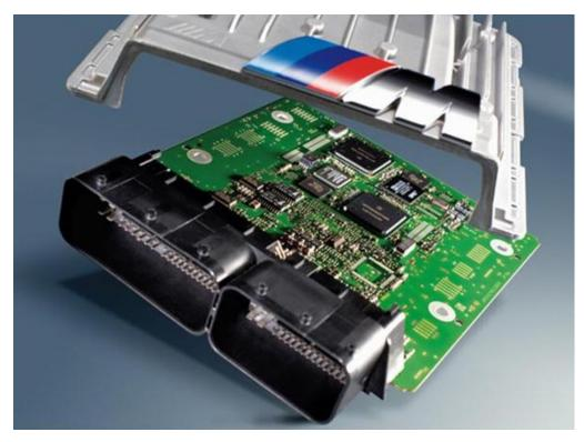
The ECM uses a multi-layer circuit board with over 1000 individual parts. There are three 32 bit processors which allow a combined capability of over 200 million engine calculations per second.
