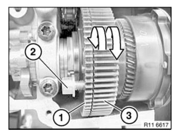
*Re-install bolt for timing chain guide rail and install timing chain tensioner. Proceed with installation of the VANOS units.*
