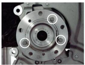
Detail of Rotor Alignment Pins on Hub
