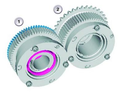
The VANOS transmissions provide the minimum and maximum "spread angle" for the camshafts. The intake camshafts have a spread angle of 60° relative to the crankshaft, and the exhaust camshafts have a spread angle of 37° relative to the crankshaft.
