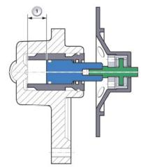
1. Stroke range of adjustment piston
