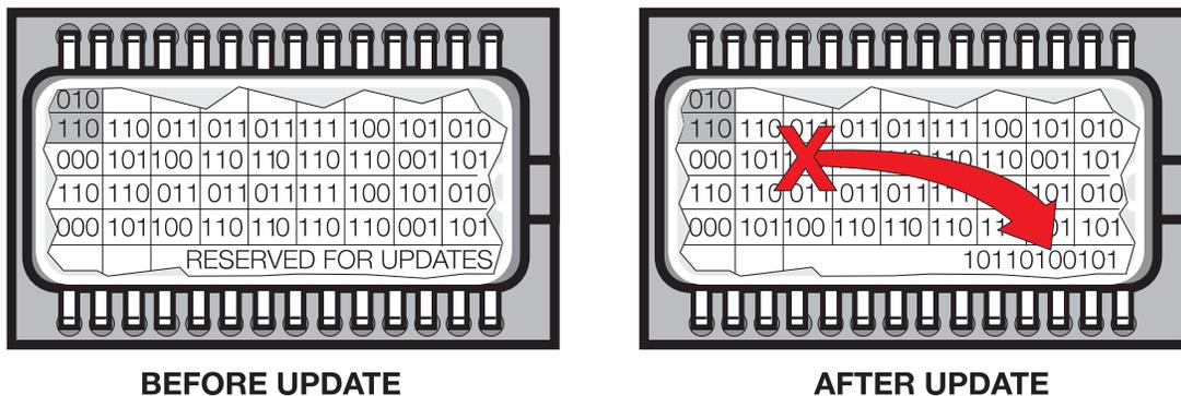
For the M3.3 & M3.3.1 systems the replacement EPROM that is installed does not contain all the data necessary for the engine to operate, it is a “basic” EPROM that only contains some basic data referred to as “resident data” which helps identify the module and allows the diagnostic equipment to determine what program and associated data needs to be installed/loaded.
