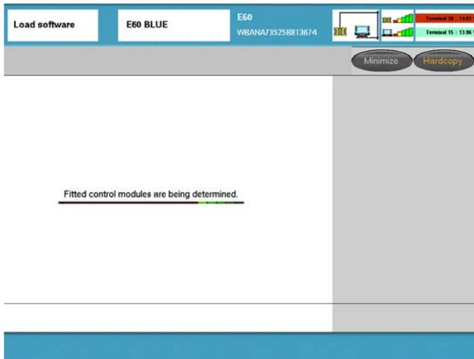
After selecting “No” CIP evaluates the installed control modules to determine if any updates are required.
