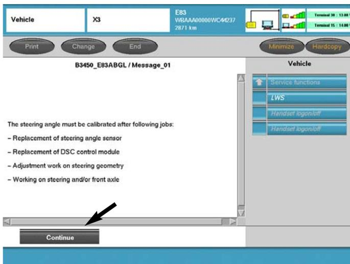
By selecting continue the process to calibrate the steering angle sensor will be carried out.
