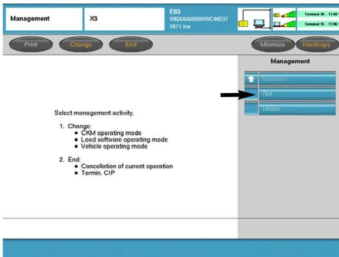
Select “**Test**” if system files are to be checked.
