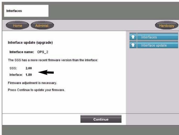
This function allows the firmware of the interface to be checked against the version of the SSS.
