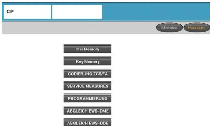
On older vehicles the Car Memory and Key Memory settings can be accessed via the SGC/UNIX function (refer to Progman Module and the section pertaining to accessing CIP Functions for E31/E32/E34/E36/E38/E39/E46/E52/E53).
