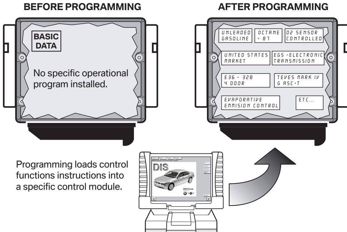
(Program) into a module/component which already has the systems operating requirements (Data) installed, plus it can be used as a means of updating data and operating instructions previously installed in a control module.
