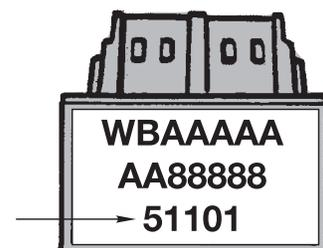
If this is no longer possible, the coding plug must be removed in order to read the code on the label of the coding plug.
