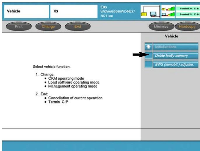
By selecting **“Delete fault memory”** the fault memory of all installed control modules will be cleared.
