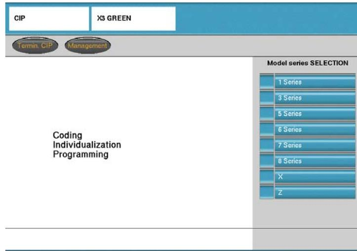
Progman incorporates all Coding, Individualization & Programming functions that were previously part of the DIS CD for E31/32/34/36/38/39/46/52 & E53, which operates under the old SGC/UNIX application, into the CIP application.
