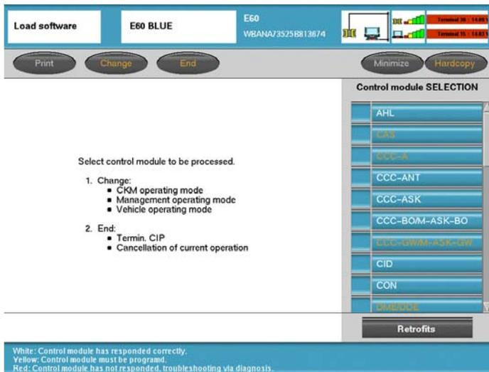
From the “Control module selection” screen specific control modules can be selected for reprogramming.
