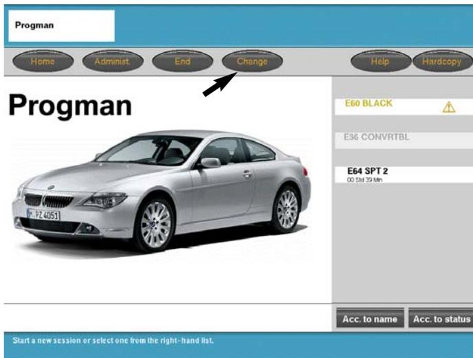
If using a GT1 it is possible to switch from Progman to a diagnostic function.
