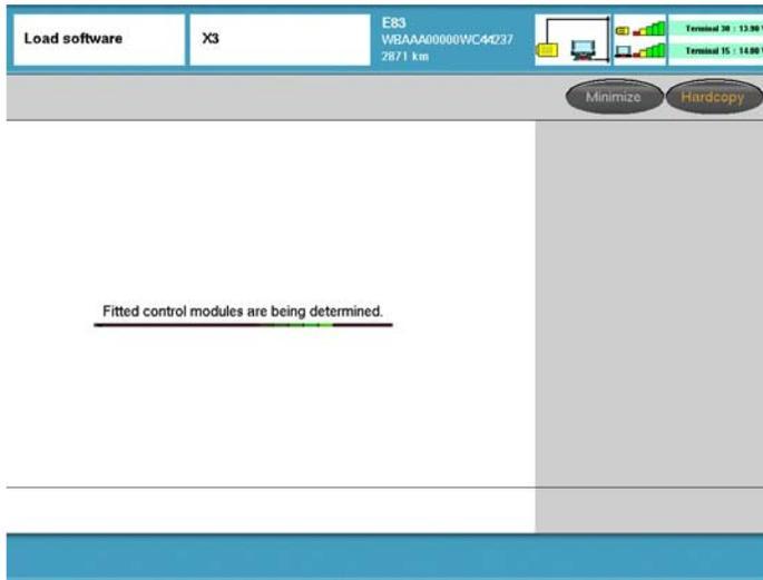
After selecting “Yes” on the Yes/No selection screen a determination/check of all installed control modules is performed.
