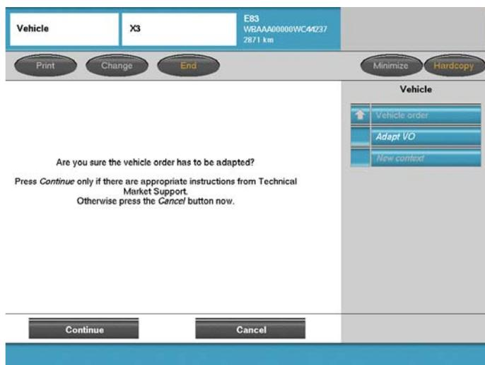
Before selecting **“Continue”** a floppy disk (1.44) containing the modified/new vehicle order must be inserted into the disk drive of the SSS.
