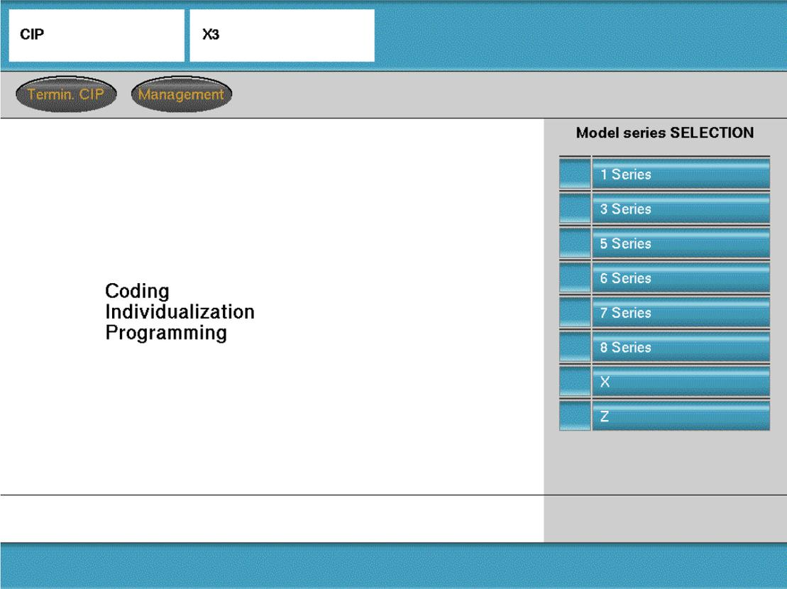
From the initial CIP screen select the model for which a coding or programming session is to be performed.
