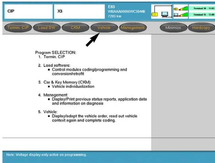
“**Vehicle**” can be selected from the main CIP selection screen to access additional functions:
