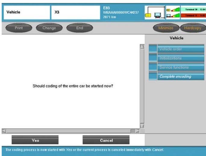
By selecting “**Yes**” all installed control modules will be recoded based on the information contained in the Vehicle Order.
