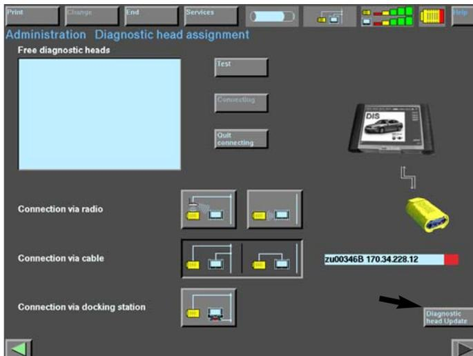
With a connection to the interface established a message should be displayed indicating that the firmware in the head needs to be updated, perform the update by selecting the “Diagnostic head Update” button.
