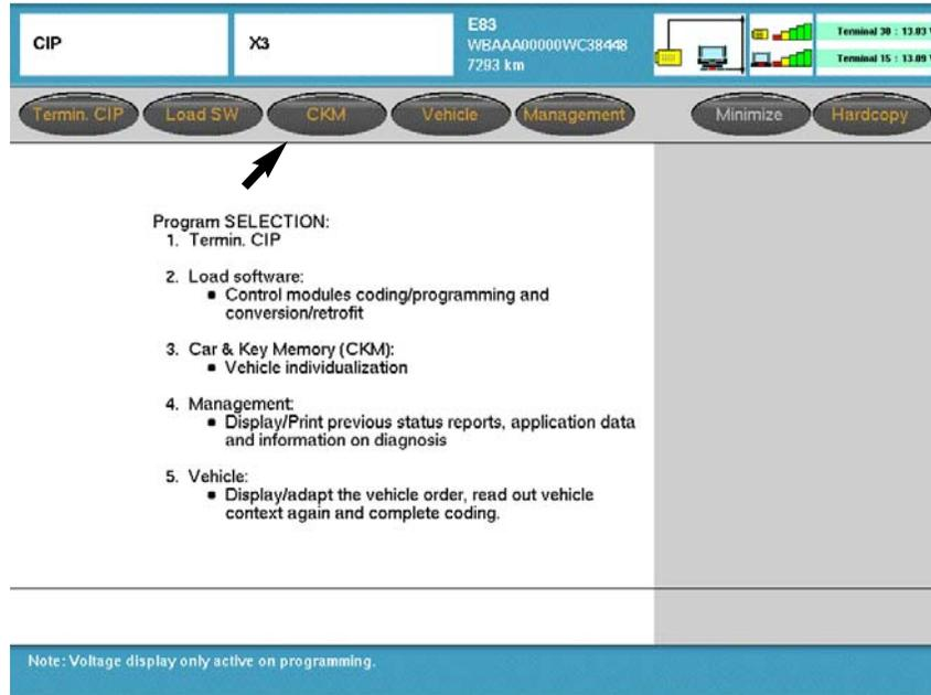
The CKM feature contained in CIP (for models produced as of the E65) provides the ability to “customize” certain vehicle and key functions to meet the specific preferences of the customer. It is important to note that the functions/features that can be “customized” will vary depending on model, equipment level and vehicle software level.
