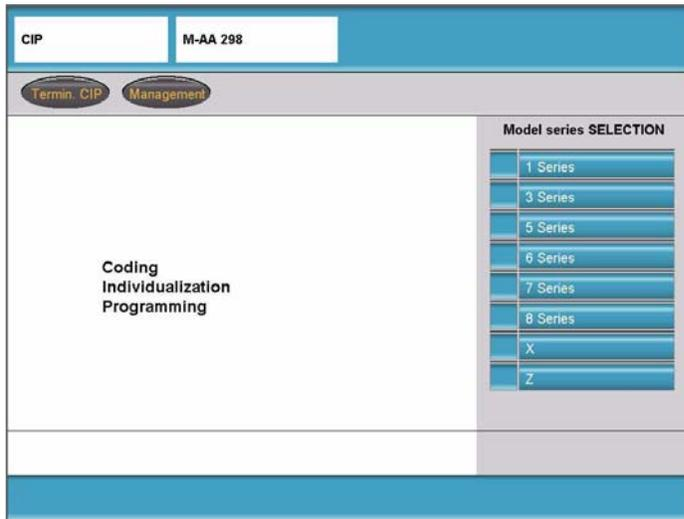
From Progman establish a connection to the interface connected to the vehicle and access CIP.
