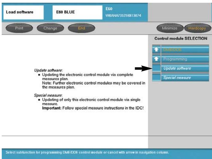
By selecting “**Update Software**” a measures plan will be generated that will indicate what updates if any are available not only for the DME but for all modules installed in the vehicle.
