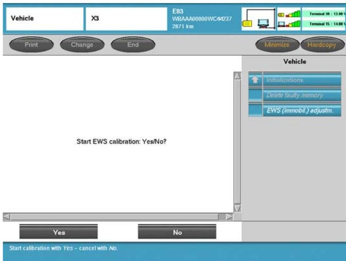
By selecting **“Yes”** the calibration/initialization of the rolling code tables in the DME and CAS or EWS modules will be carried out.
