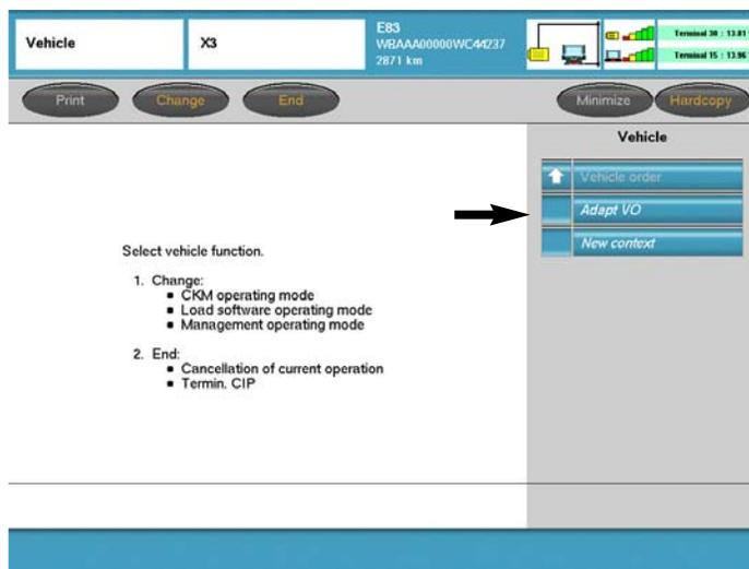
Selection of **“Adapt VO”** provides the ability to install a modified Vehicle Order file.
