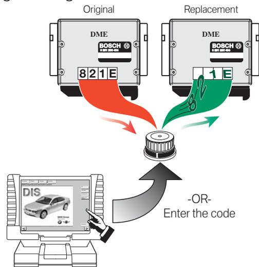
**Note: M1.X DME control modules can only be coded up to eight (8) times. The GT1/DISplus will display the remaining number of times the control module can be recoded.**
