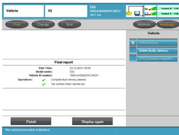
Displays a report pertaining to the clearing of the fault memory on all installed modules.
