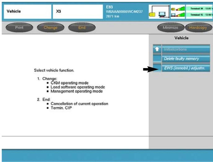
By selecting **“EWS adjustm.”** or **“CAS Calibration”** the rolling code tables can be initialized.
