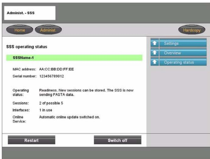
**This is the only location from which the SSS should be restarted or shutdown using the buttons at the bottom of the screen.**
