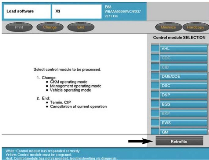
Select **“Retrofits”** to view a list of functions/features that can be modified or installed.
