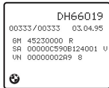
**Note: As of 9/98 production the ZCS label was eliminated from the vehicle. Some older vehicles will have identification labels containing an AM segment, this information is not needed for coding or recoding a control module on that vehicle.**
