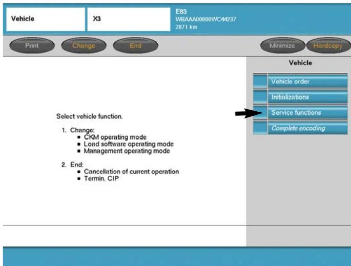
The **“Service function”** feature provides access to various calibration functions.
