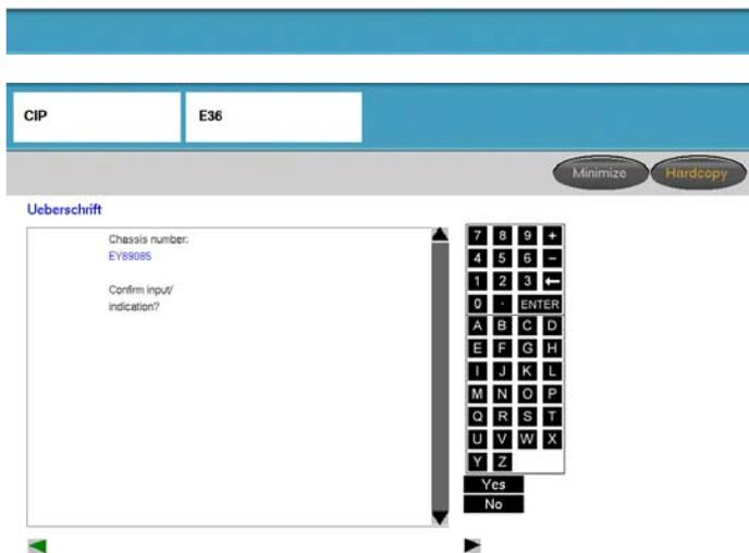
Chassis number of vehicle is displayed, enter VIN using touch screen pad or the keyboard on an SSS.
