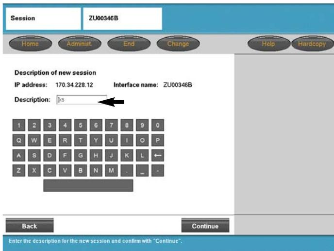
Under "Description" enter information that will identify the vehicle to which the interface is connected (Ex. VIN or Model type, Service hat #, Vehicle color, Bay location, etc.)
