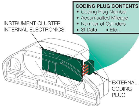
By using a plug that is able to store data, the instrument cluster can be replaced without losing vehicle mileage, unless the coding plug is damaged.
