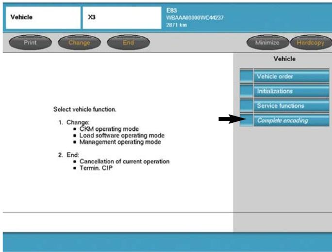
“**Complete encoding**” provides the ability to code/decode all control modules installed in the vehicle.
