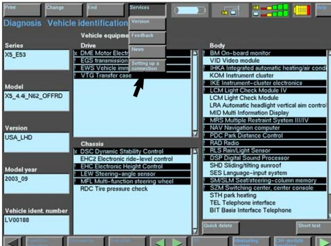
If the vehicle to be programmed was previously being diagnosed using a diagnostic head with the GT1, then the connection with the head must be broken before that head will be recognized by Progman.
