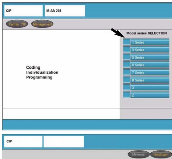
From Progman establish a connection to the interface connected to the vehicle and access CIP.
