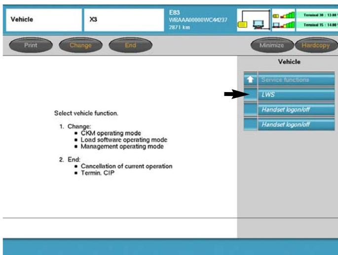
Selecting **“LWS”** will provide the ability to calibrate the steering angle sensor.
