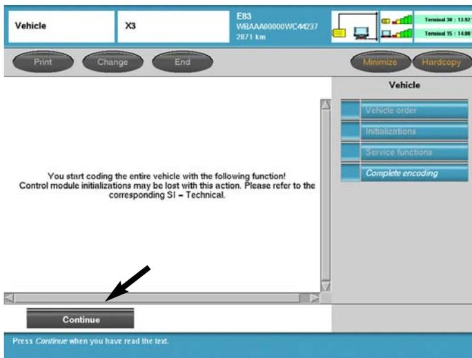
Recoding all the installed control modules may result in the loss of initialization or system settings such as radio station presets or seat/mirror memory.
