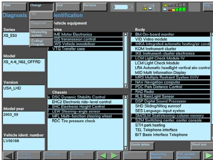
If using a GT1 it is possible to switch from a diagnostic function to Progman to check the status of an active session.
