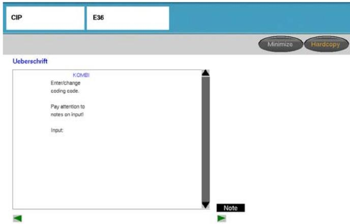
If the ZCS code must be changed follow the instruction given on screen and enter the required information exactly as indicated on the ZCS label or printout of ZCS code before removal of module.
