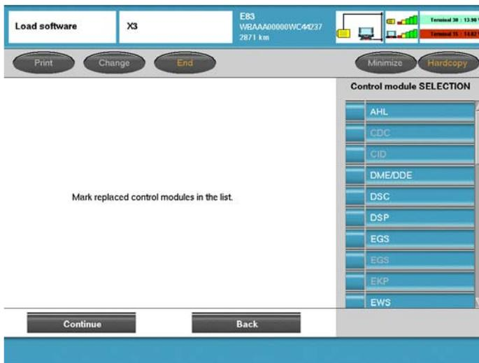
Upon completing a check of the installed control modules, a list highlighting the installed control modules is displayed.
