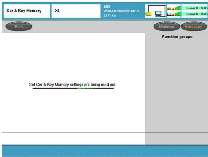
Upon selecting “**CKM**” a check of the current vehicle and key settings is made.
