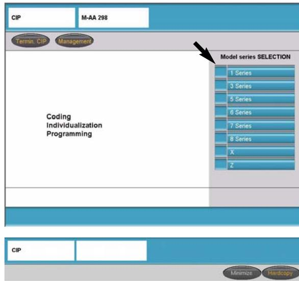
From Progman establish a connection to the interface connected to the vehicle and access CIP.
