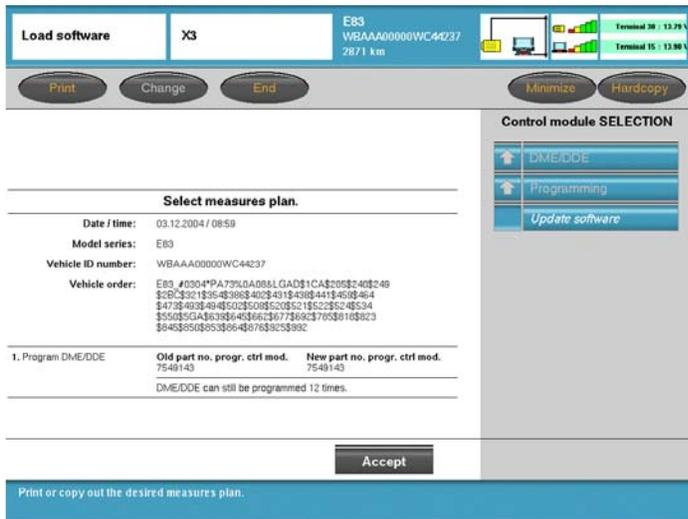
A measures plan for the selected system/module is displayed.
