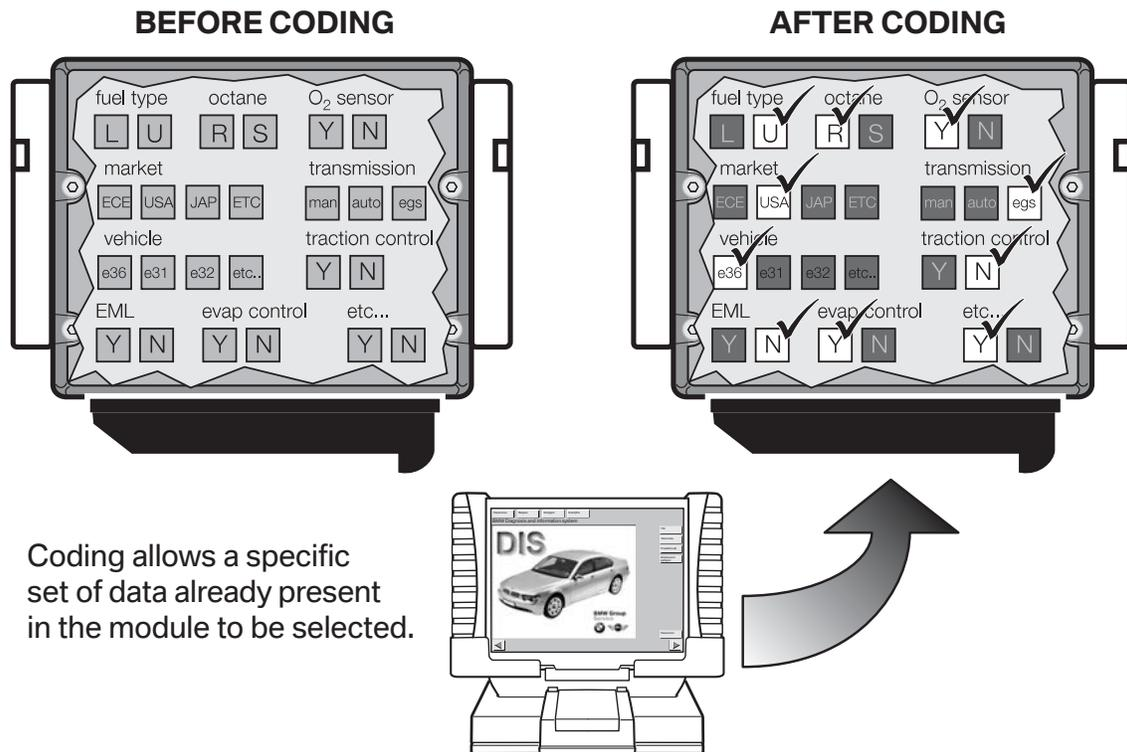
A “codable” control module has a basic operating program already installed along with several specific variations of operating data. The coding process allows a specific set of operating data to be assigned to the basic operating program of that module/component, with respect to its specific application.
