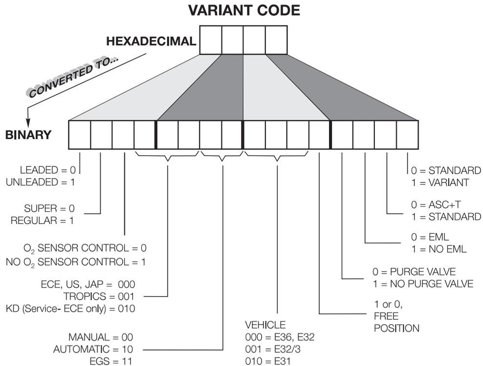
Under no circumstances should the variant code to be changed from the assigned number for the vehicle. Erratic engine operation and possible engine damage may result.
