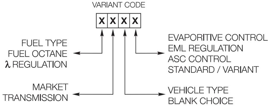
The information from the variant code is used to define the the operational data to be assigned to the operating program of the module.
