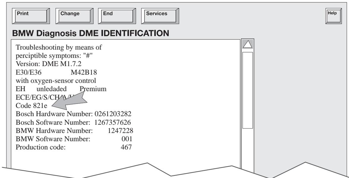
If a control module malfunction is suspected cross reference the BMW and Bosch part numbers in the display with the installed variant code. Problems can occur if:
