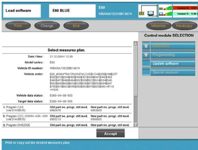
A "Measures plan" provides information on updates that are available for all installed control modules. By selecting accept, all modules listed in the measures plan will be updated.
