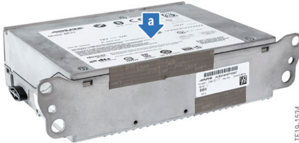
Head Unit High 3 Flash (HU-3_F) (with eMMC flash memory)
