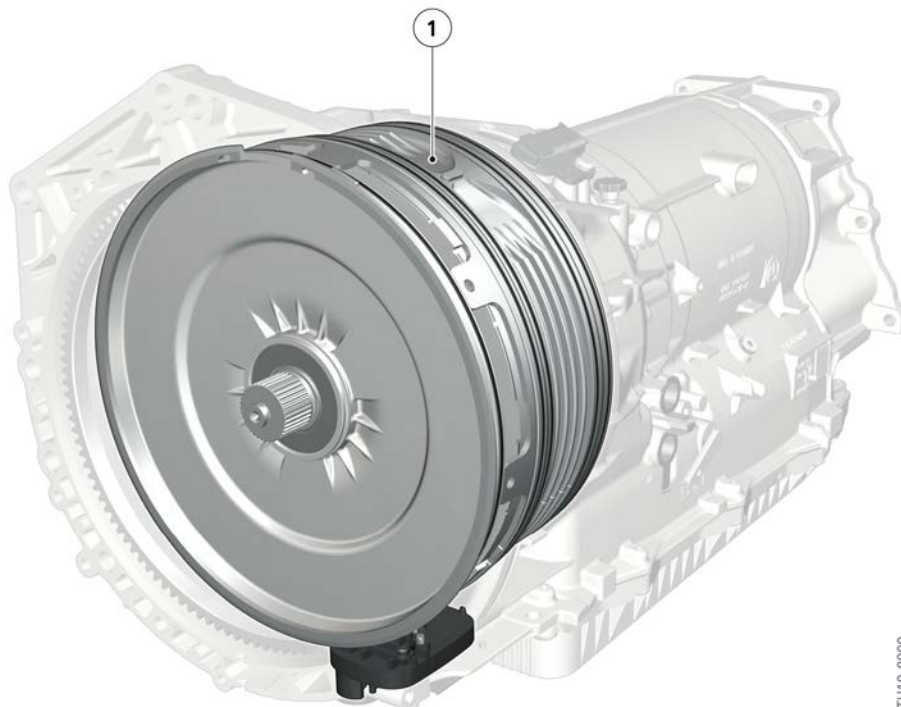
Electrical machine in the GA8P75HZ transmission
