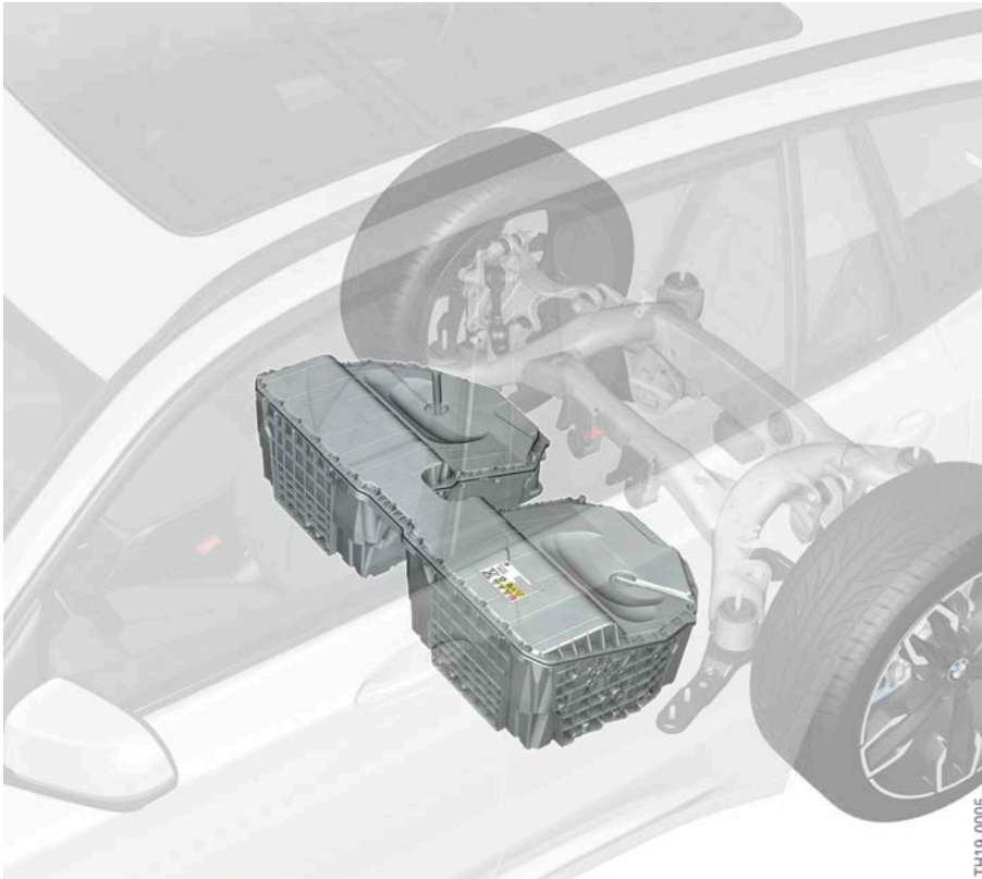
G01 PHEV, installation location of the high-voltage battery unit
