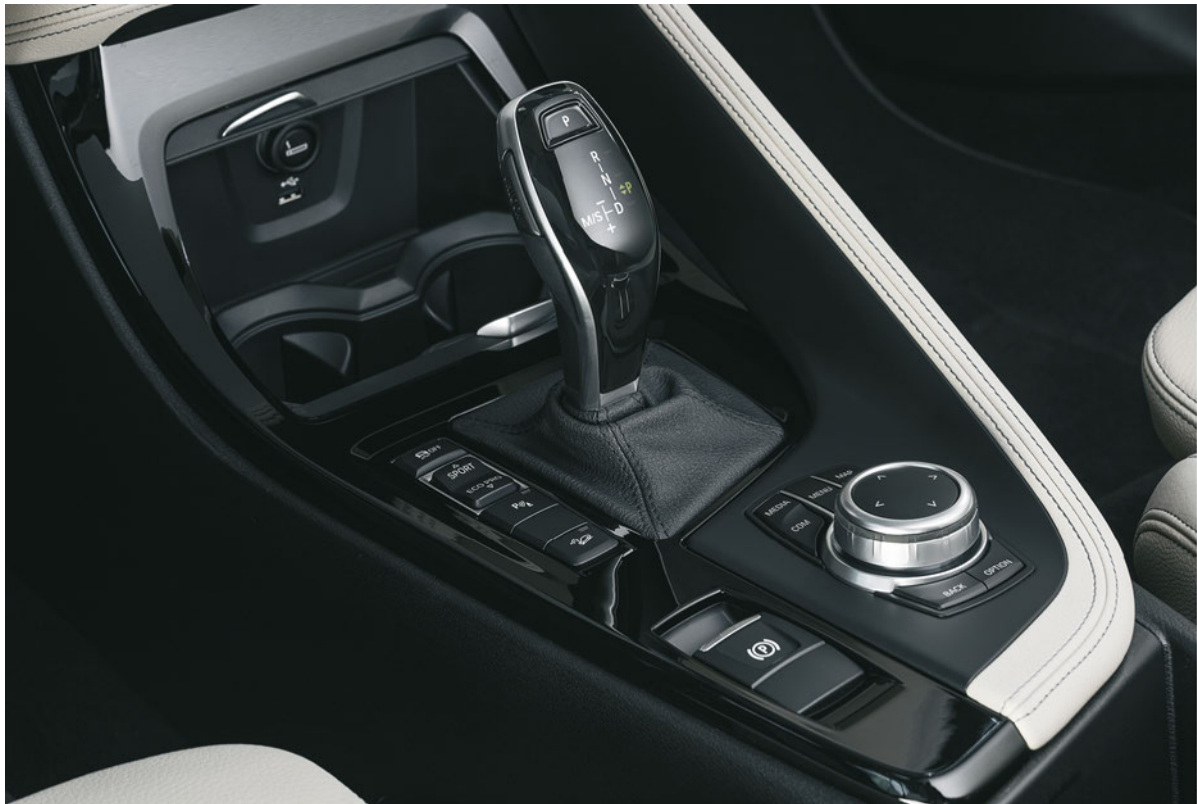
Gear selector switch
