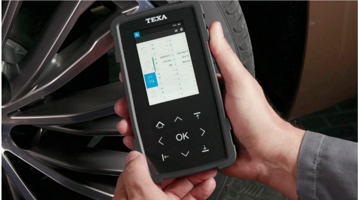
Reading out the wheel electronics with the RDC Tool
