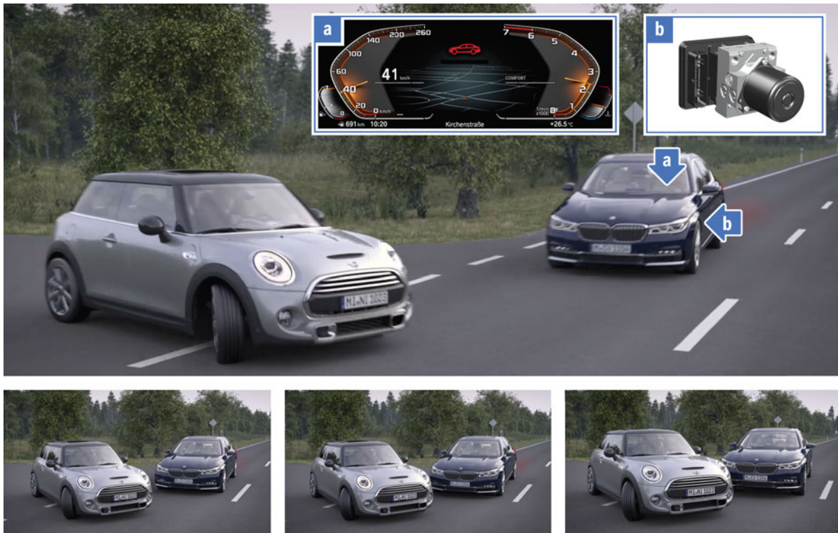
Intersection collision warning
