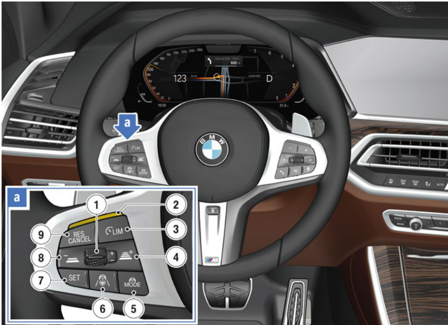
Control panel for assistance systems at the multifunction steering wheel (with optional equipment "Active Driving Assistant Professional" (SA 5AU))
