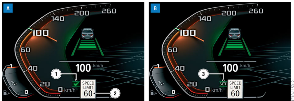
Displays in the instrument cluster when Speed Limit Assistant is activated (automatic and manual)
