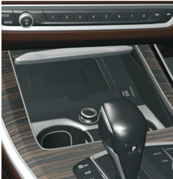
Wireless charging station
