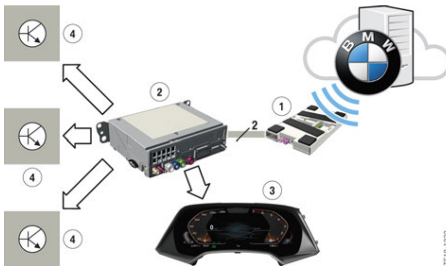
Remote Software Upgrade data distribution
