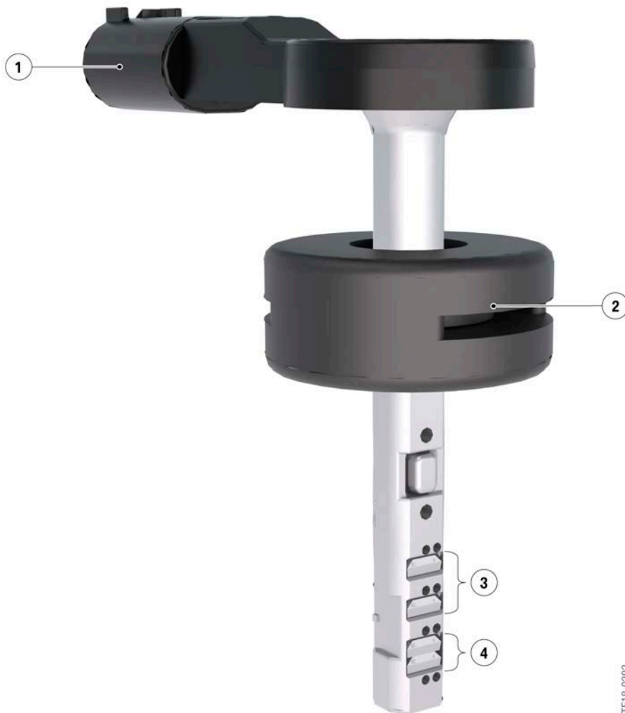
Brake fluid level sensor with Hall effect sensor
