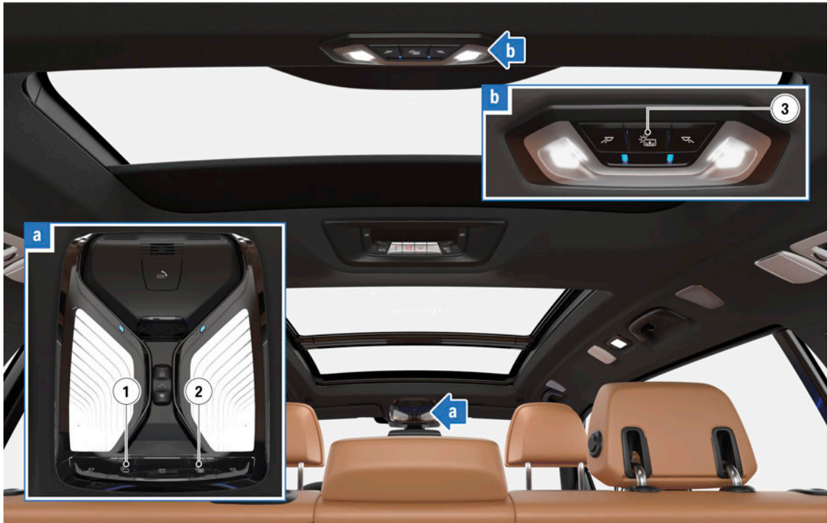
Control of panoramic sunroof roller blind for 3rd row of seats
