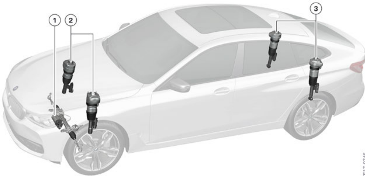
G32 Adaptive two-axle ride level control
