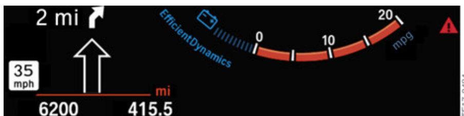
Display of speed limit info in the extended and enhanced instrument cluster
