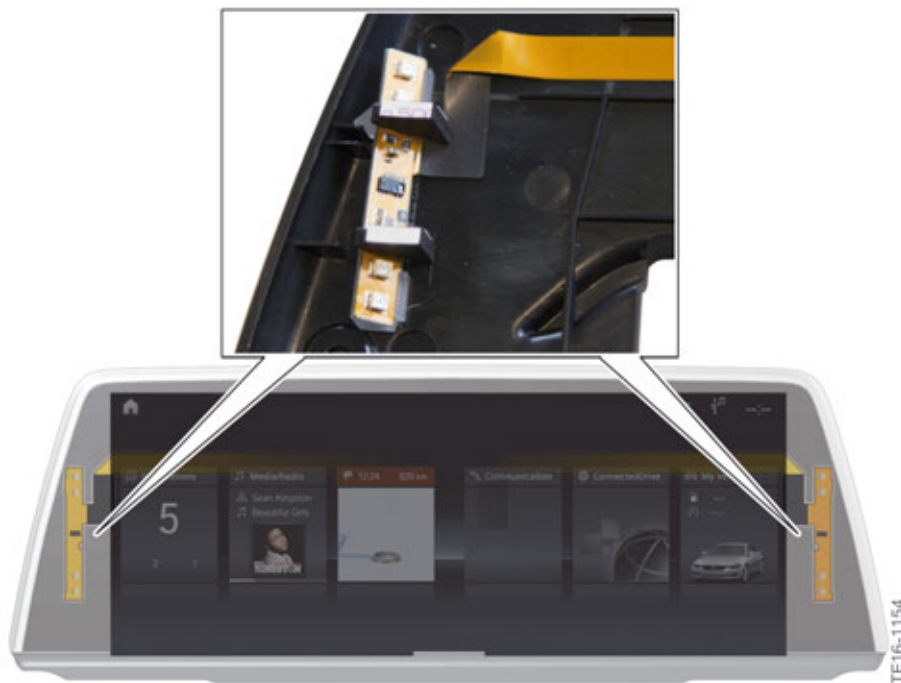
F22/F23/F87 LCI infrared sensors for the central information display (CID)
