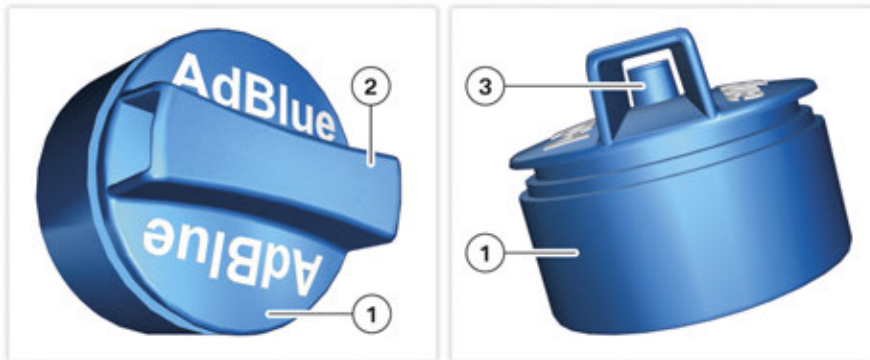
SCR 3, urea/water mixture (AdBlue®) fuel filler cap
