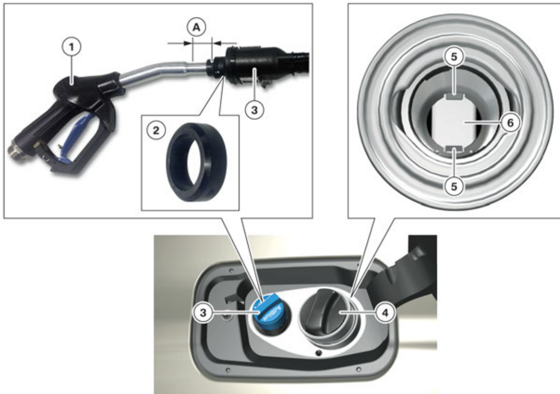
Misfilling protection in SCR filler neck and diesel filler neck (ECE G12 shown).
