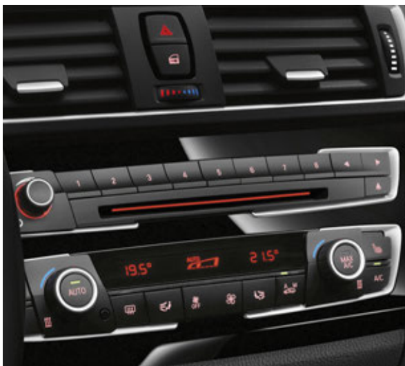
F34 LCI air conditioning control panel
