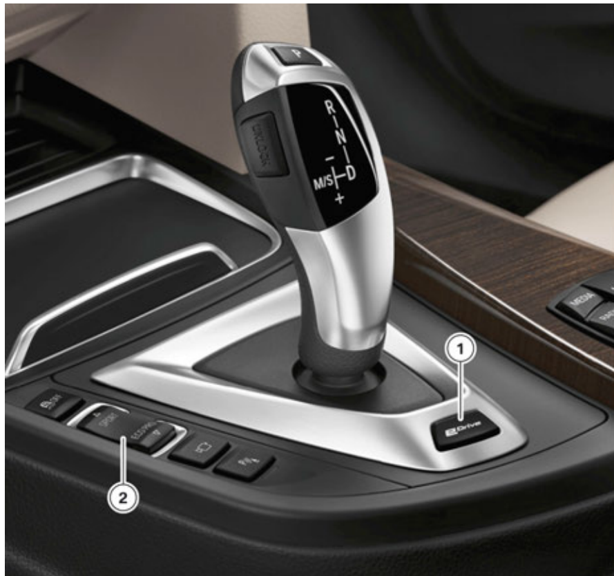
F30 PHEV eDrive button and driving experience switch
