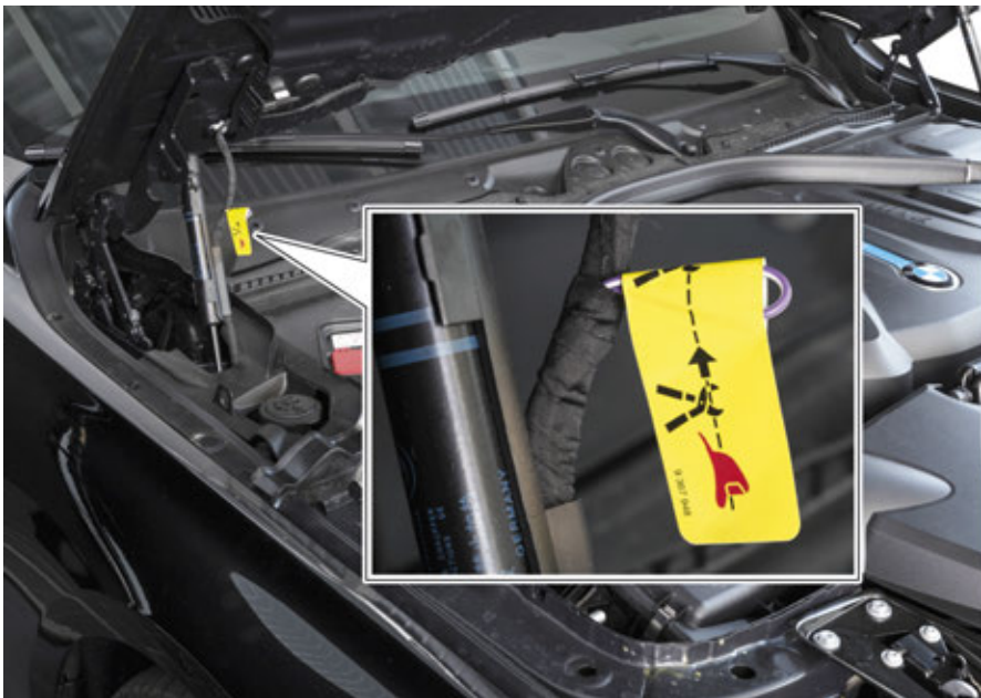
F30 PHEV, installation location of emergency separation point
