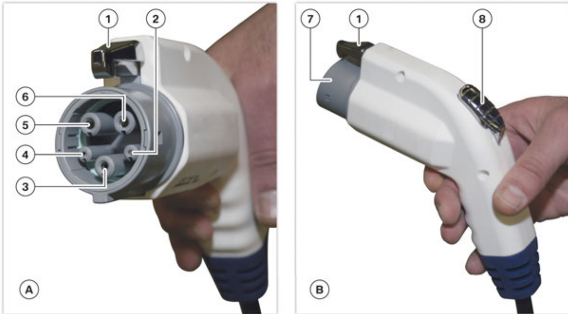
F30 PHEV, Connector of the charging cable for the connection to the vehicle (standardized i.a.w. IEC 62196-2: Type 1)
