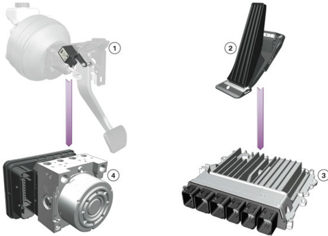
F30 PHEV, components for input signals of brake energy regeneration
