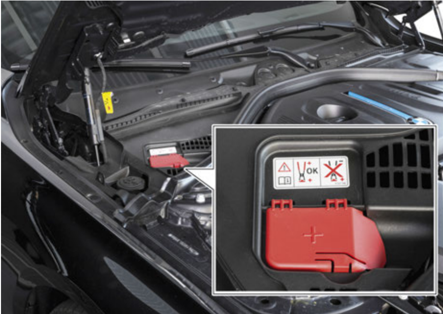
F30 PHEV, positive battery connection point
