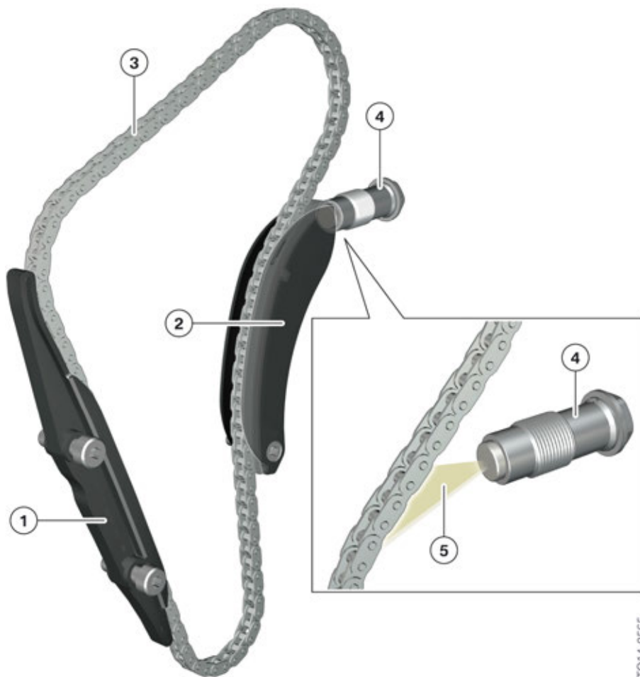
Lubrication of top chain drive, B46 engine
