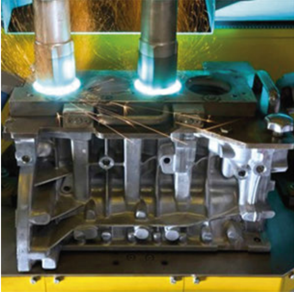
Electric arc wire spraying method, Bx8 engine
