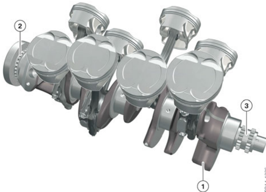
N63TU2 engine, crankshaft drive with connecting rod and piston
