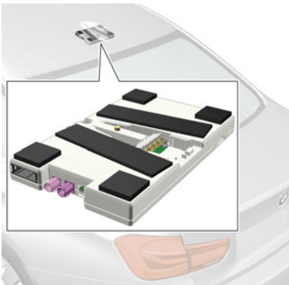
Installation location of Telematic Communication Box 2 (TCB2) in F30 LCI
