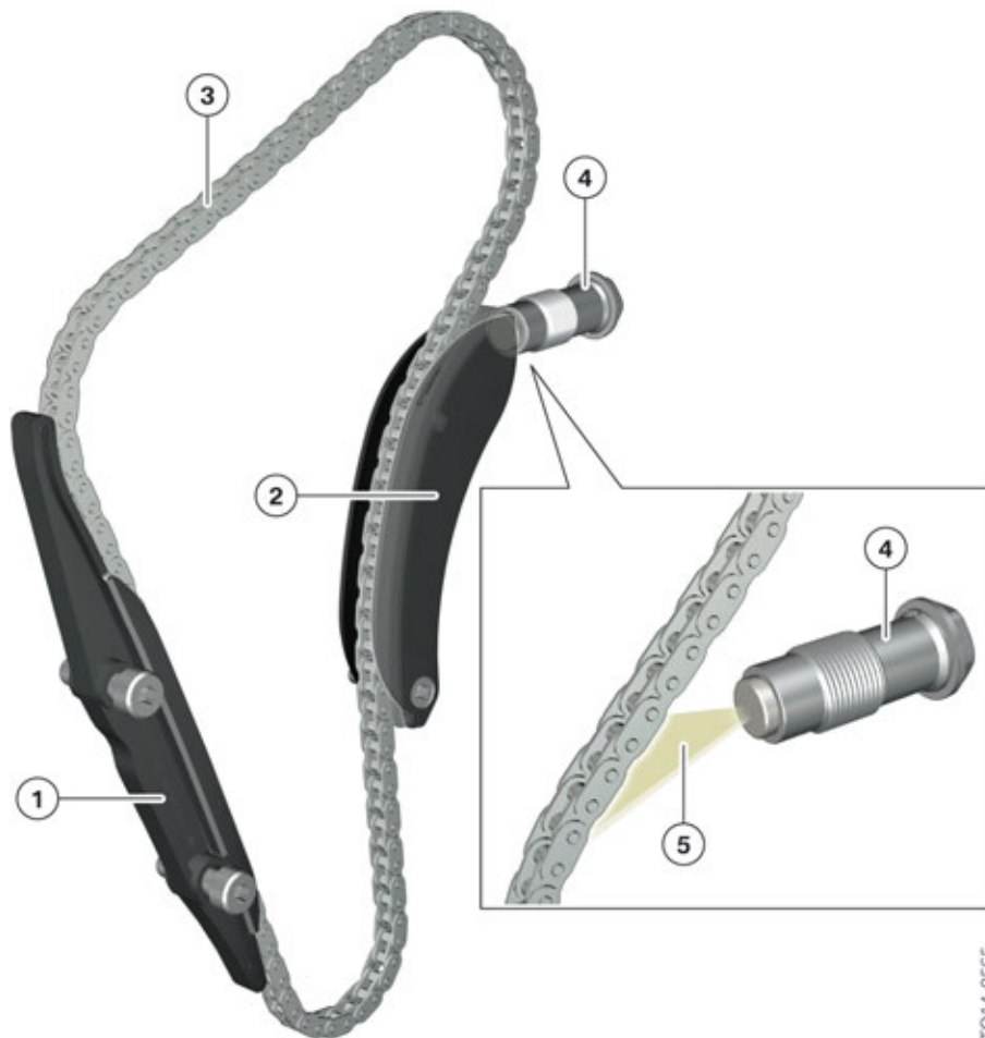
Lubrication of top chain drive, B38 engine
