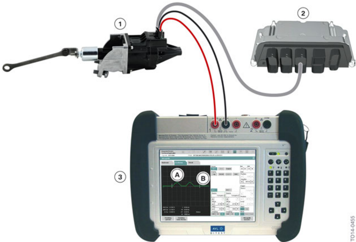
Sensor signal to electrically adjustable wastegate valve
