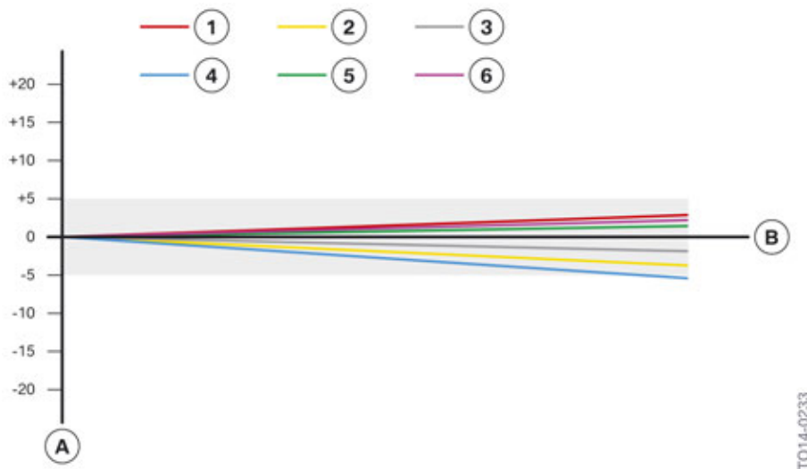
S55 engine, injector, minimal quantity adjustment with CVO
