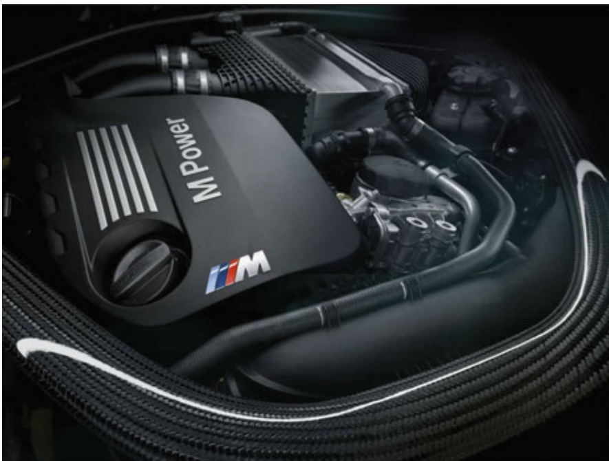
F80/F82 air intake duct and indirect charge air cooler
