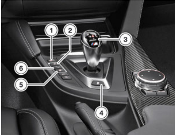
F80/F82 M DCT Drivelogic gear selector switch and driving dynamics button
