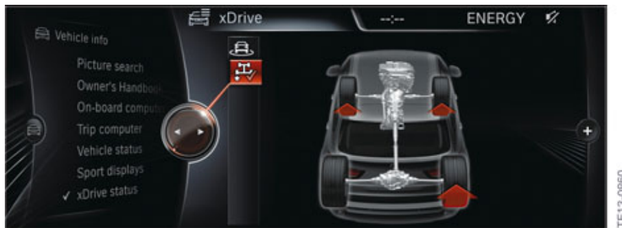
F15 display of drive torque distribution xDrive in the central information display
