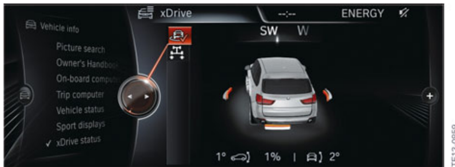
F15 status display of xDrive in the central information display
