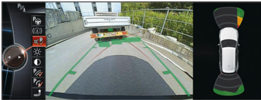
Schematic diagram of reversing camera in the CID
