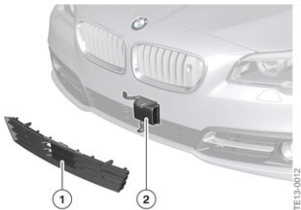
BMW 5 Series LCI Installation location of radar sensor
