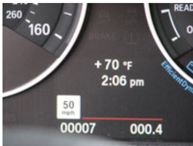
Speed limit information displayed on the instrument cluster (F30 graphic shown)
