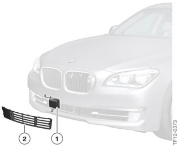
F01/F02 LCI - Installation location of radar sensor
