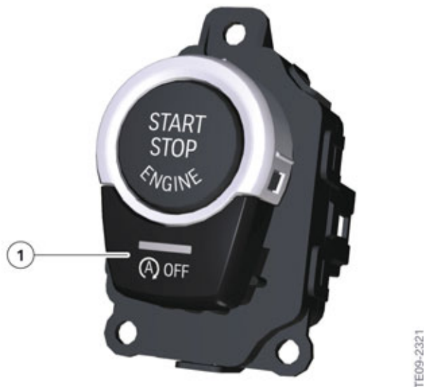
F01/F02 LCI automatic engine start-stop function button
