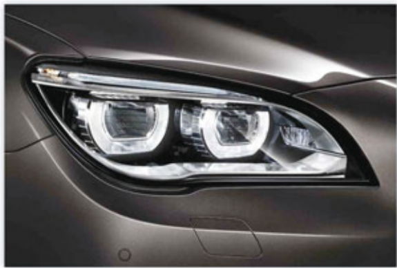
F01/F02 LCI low-beam headlight of the LED headlight
