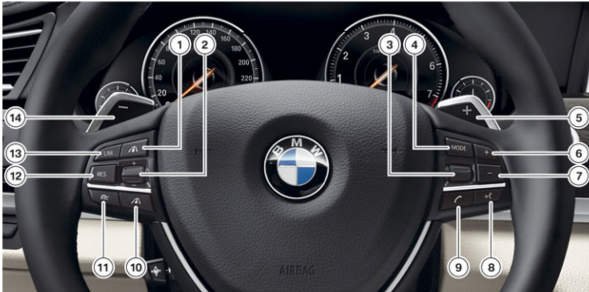
F01/F02 LCI operating controls on the steering wheel
