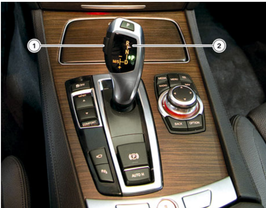
Electronic transmission emergency release GA8HP
