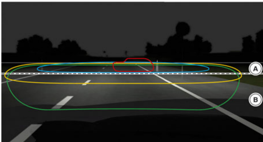
F01/F02 LCI light distribution of the LED arrays of the LED headlight
