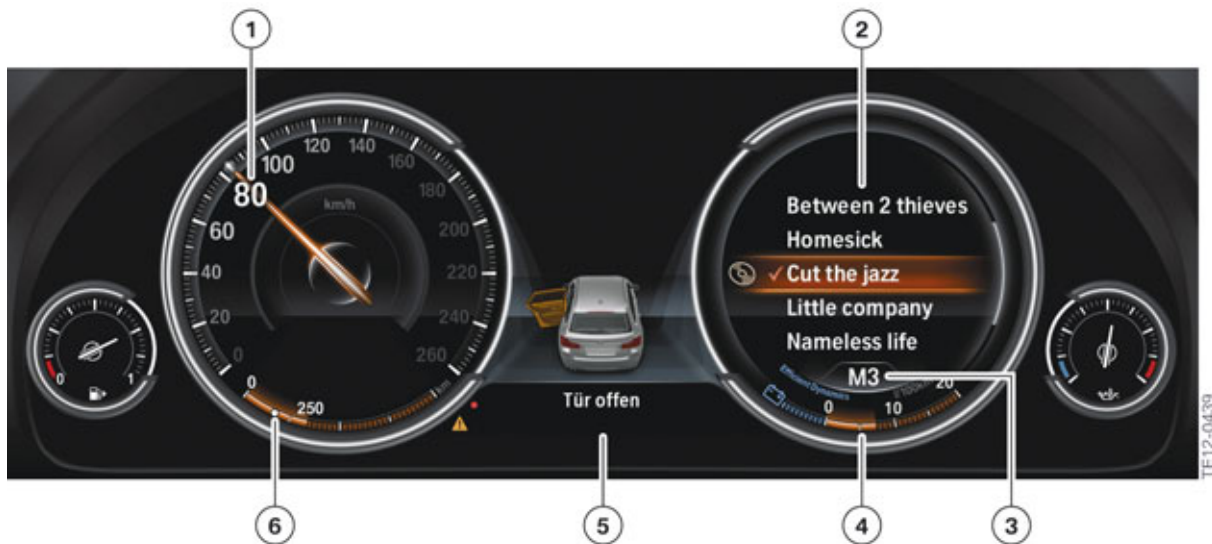
Sample display of dynamic digital instrument display
