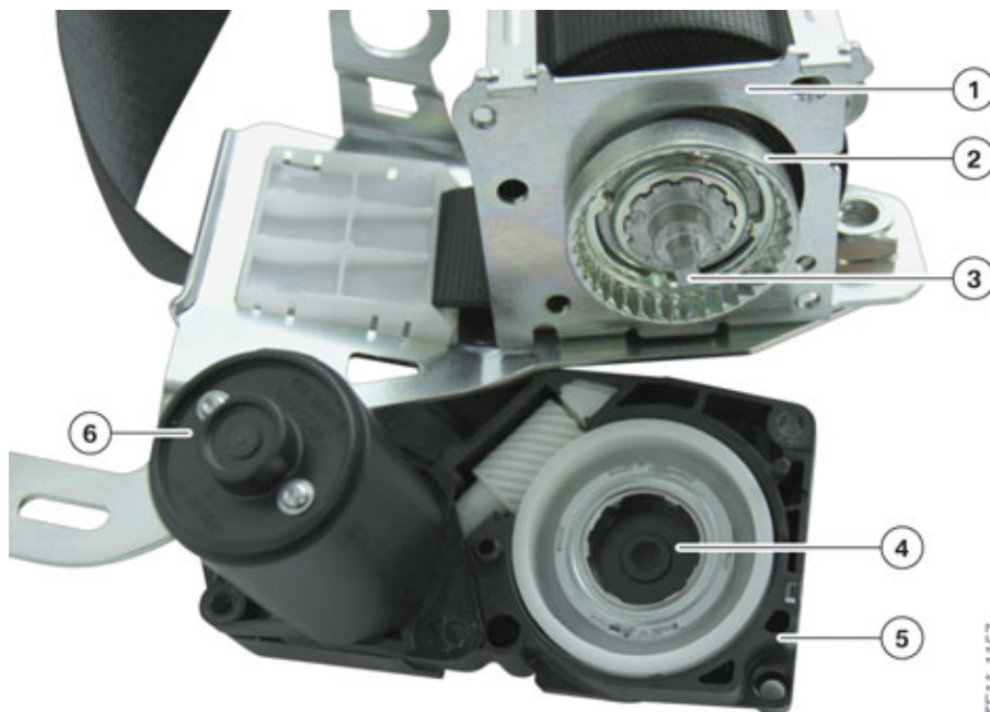
Structure of reversible motor-driven reel
