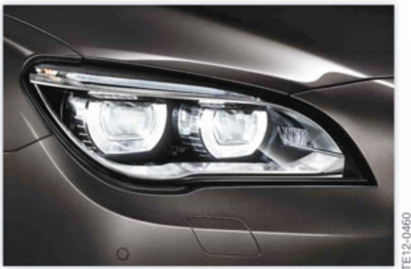
F01/F02 LCI high-beam headlight of the LED headlight
