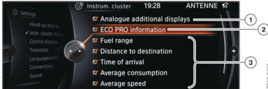
Switching on/off changeover of displays
