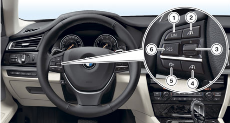
F01/F02 LCI - Steering wheel, ACC Stop & Go
