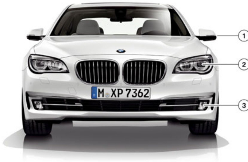
F01/F02 LCI exterior lights at front with adaptive LED headlight
