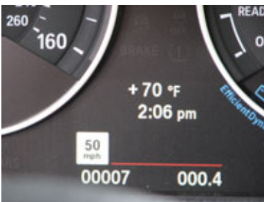
Speed limit information displayed on the instrument cluster (F30 graphic shown)
