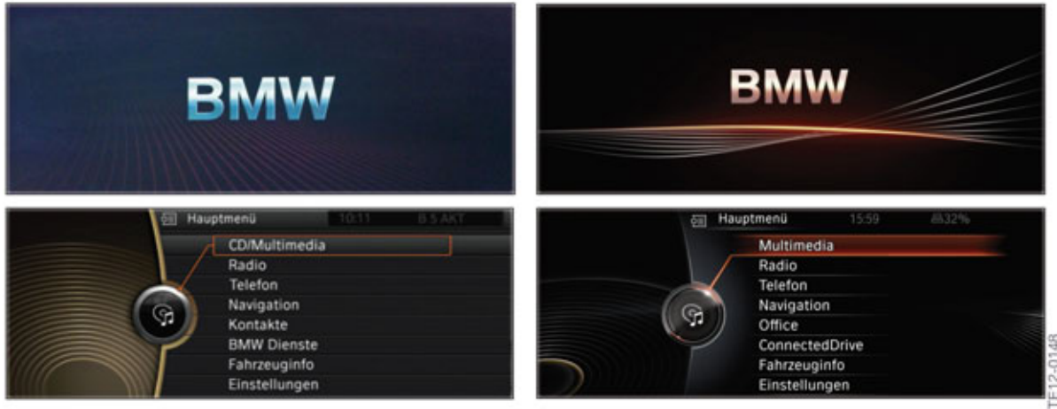
Main menu and start screen; comparison of CIC (left) to Headunit High 3rd Generation HU-H (right)
