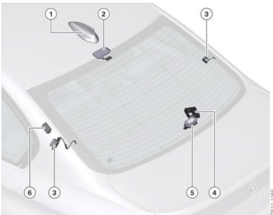
F30 Antenna system
