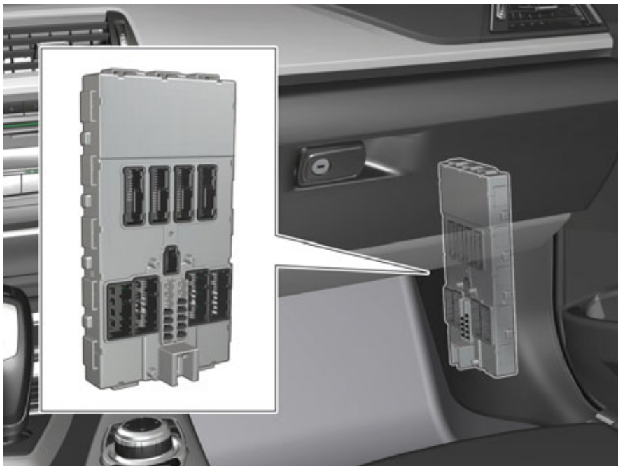
F30 FEM installation location
