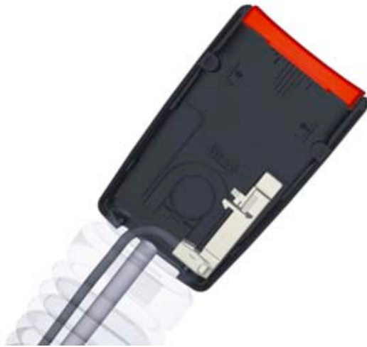
F30 Seat belt buckle switch
