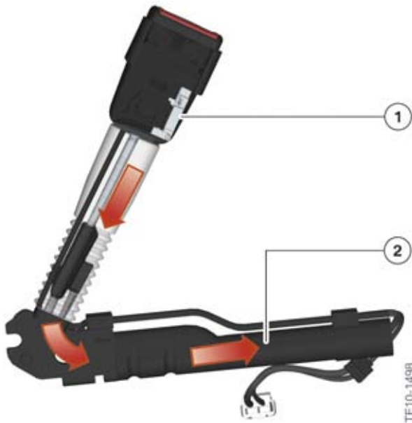
F30 Seat belt buckle tensioner
