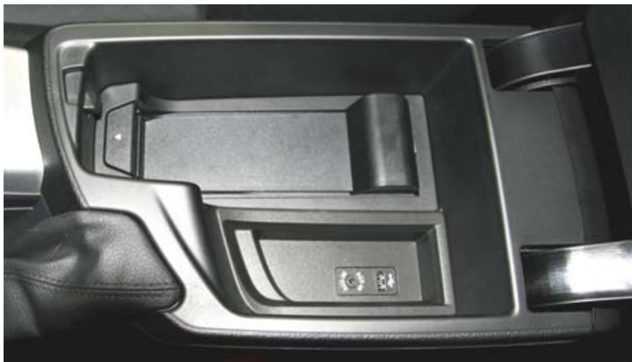
F30 mobile phone preparation with AUX-In connection with USB audio interface
