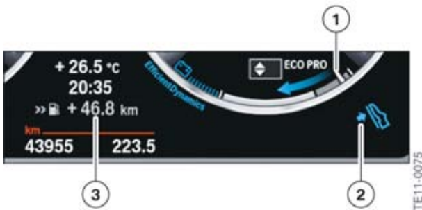
Displays of the ECO PRO mode in the instrument cluster with extended functional scope (extended cluster function optional equipment 6WA)
