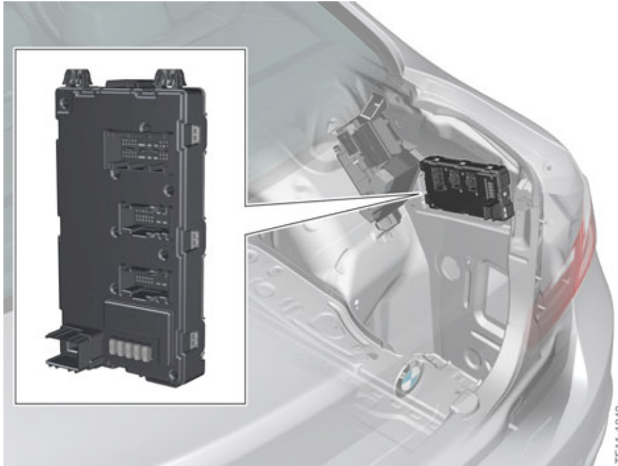
F30 REM installation location
