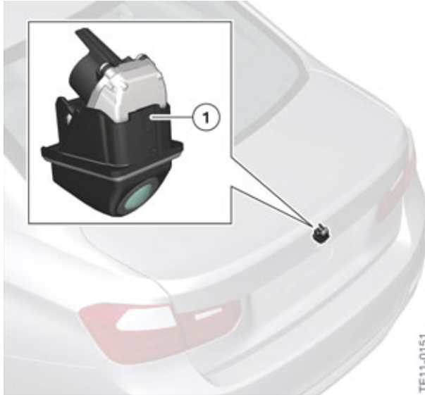
Installation location, reversing camera
