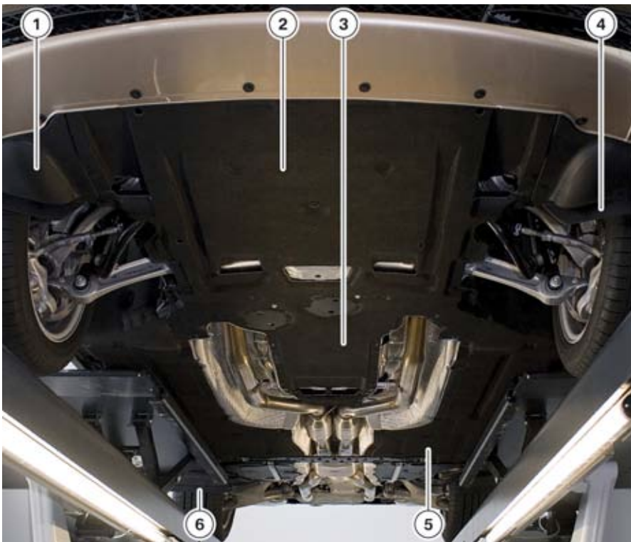
F10 Underbody panels (aerodynamic measures)
