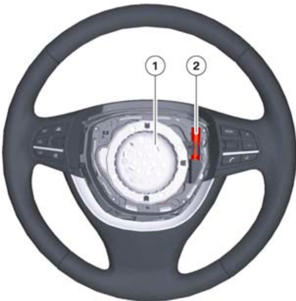
F10 Adaptive Driver's airbag steering wheel with the airbag removed.
