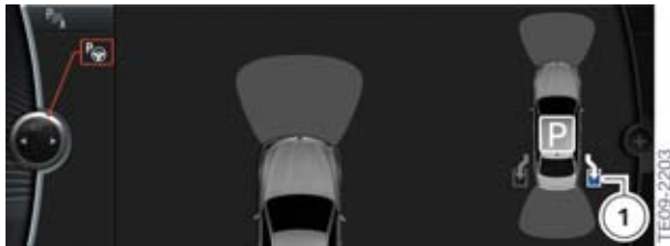
F10 Parking display when parking assistant is not activated, with parking space found to the right
