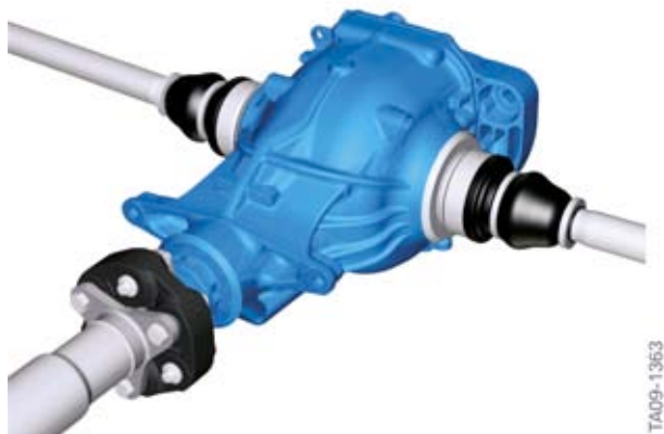
F10 Rear axle final drive lightweight construction
