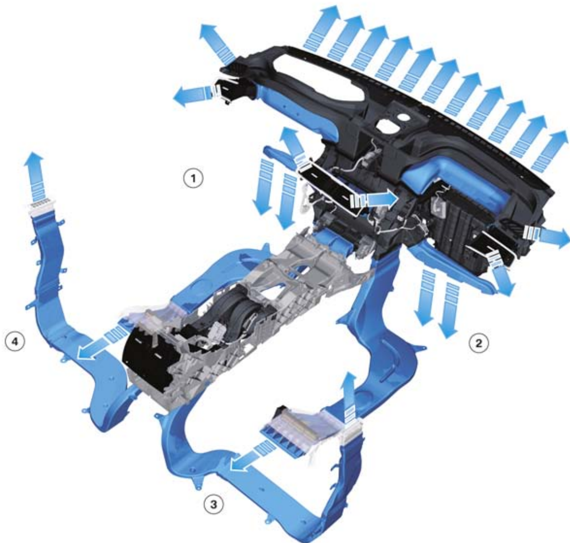
F10 Air ducts and zones of the 4-zone IHKA
