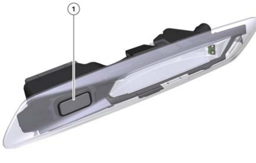
F10 parking assistant ultrasonic sensor in the right side marker turn signal indicator
