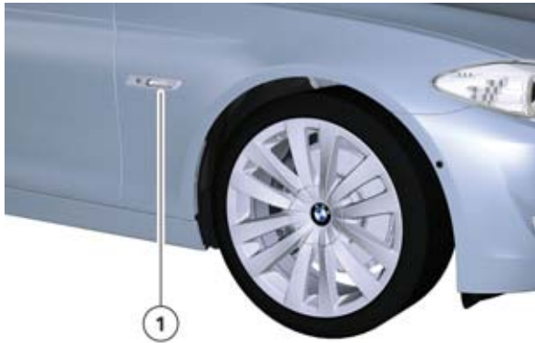
F10 Installation location of the parking assistant ultrasonic sensor in the side marker
