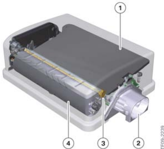
F10 Structure of the sensor for ACC Stop & Go.
