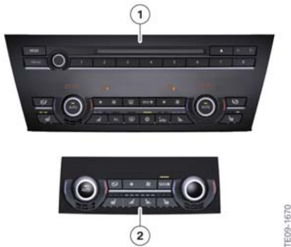
F10 Control panels for the 4-zone IHKA
