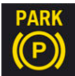
F10 Indicator light, parking brake fault display
