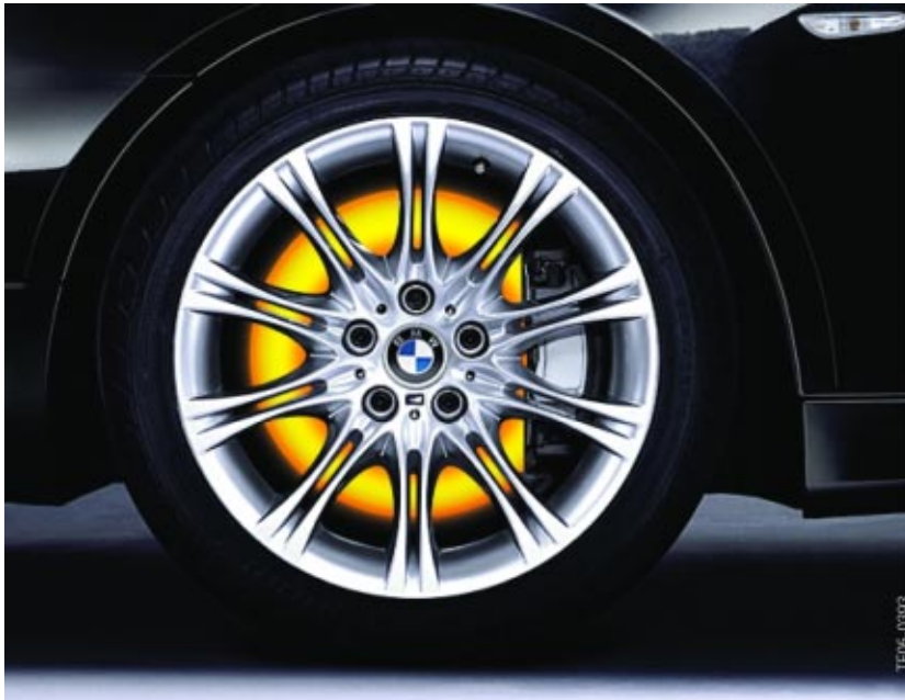
Brake Disc with Fading
