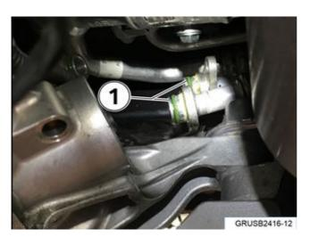
11. Replace the O-rings on the transmission cooler lines (from transmission cooler) (1).
