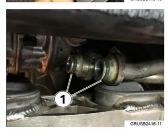
10. Replace the O-rings on the transmission cooler lines (from transmission) (1).
