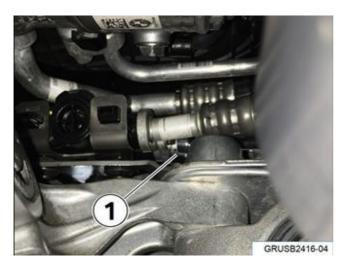
b) (access from under the car) feed the socket/extension up over the front sub-frame and attach the socket to the bolt holding the cooler lines to the transmission thermostat on the cooler side (1).
