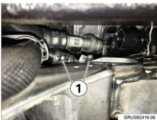
12. Tighten down the thermostat bracket bolts (1) to 8Nm.
