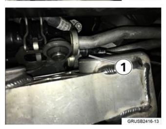
13. Tighten down the retaining bolt (1) for the cooler lines on the transmission side to 8Nm.
