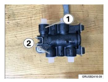
8. Install the new thermostat to the bracket.
