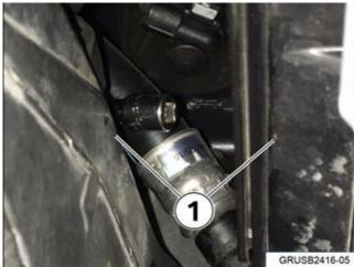
c) Attach a ratchet to the socket extension from over the subframe by the radiator (1) and remove the bolt for the cooler lines.
