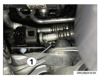
14. Tighten down the retaining bolt (1) for the cooler lines on the cooler side to 8Nm.
