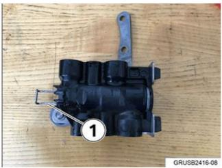
7. Undo retaining clip (1) and remove the old thermostat.
