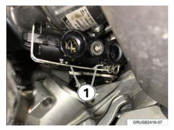
b) (Access from under the engine compartment) Rotate and pull out the transmission cooler thermostat with bracket (1).
