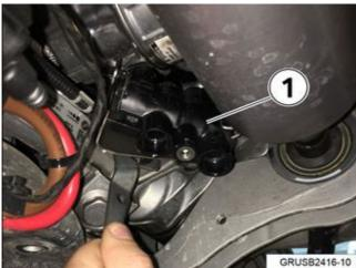
9. Attach the bracket (1) to the new thermostat before installation.
