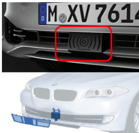
Installation location of radar-based sensors
