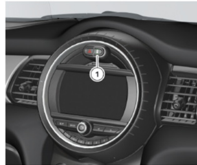
Setting of warning response time or de-activation of driver assistance systems (MINI).
