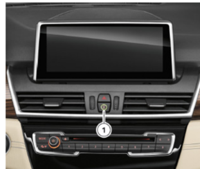
Setting of warning response time or de-activation of driver assistance systems (BMW).
