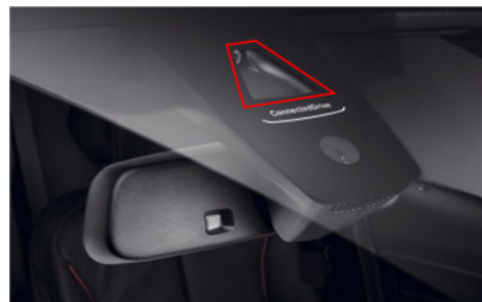
Installation location of KaFAS camera
