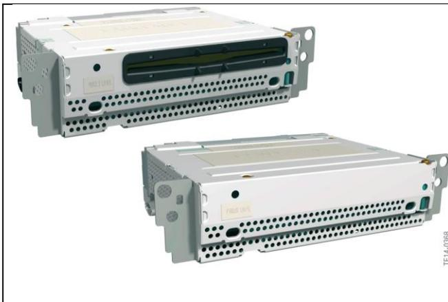
In addition, there is also a GPS module and a connection for the GPS aerial in the HU-B with Navigation.
