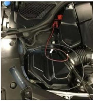
Some vehicles have a service flap in the wheel arch which can be used to route the charging cables into the engine compartment.
