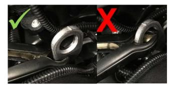
One exception is the Z4 (G29, from model year 2019). To close the hood completely with charging cables connected, the black charging clamps for terminal 31 (ground) must be connected elsewhere.
