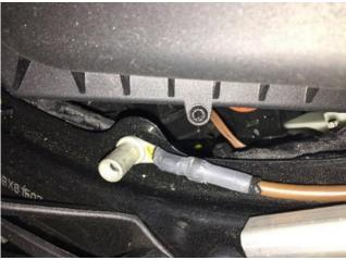
The negative lead must be connected to the jumpstart connection point or to the hook for removing the engine. The batteries must be fully recharged.
