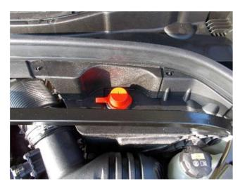
Vehicles whose batteries are installed in the luggage compartment have a connection point with a **red** protective cap featuring a "+" in the engine compartment. The positive lead of the charger must be connected to this.
