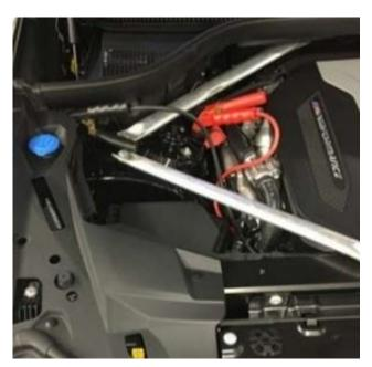
Cable routing through the engine compartment is illustrated in this example of an X5.
