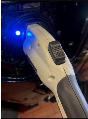
HV charging plug blue LED indicating charging
