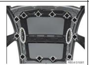
Remove the rear sunroof glass panel following repair instructions REP 54 13 250 "Removing and installing/replacing rear glass slide/tilt sunroof panel". The front glass slide/tilt sunroof will be removed at the same time.
