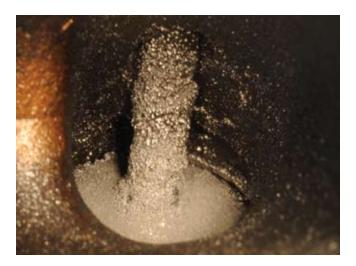
Before cleaning: Over time, even nationally known brands can leave excessive carbon deposits in the intake manifold and, especially, on the intake valves.
