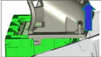
Lift the protective cap off the connector
