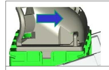
Slide the protective cap in the direction of the lock lever
