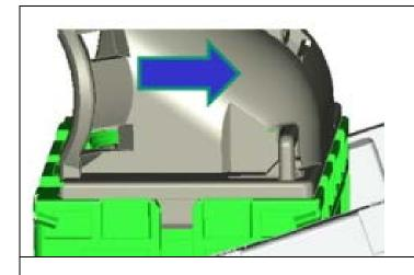
Slide the protective cap in the direction of the lock lever
