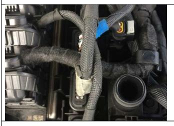
2h. Wrap the wiring harness with repair tape (P/N 61 13 6 920 760) up to the connector and reassemble.
