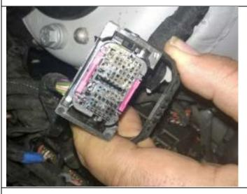
1d. Check for water residue or corrosion in the connector and in the connector chamber of the DME control unit (photo below).
