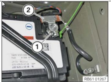
1a. Slacken nut (1) and detach battery earth lead from battery.
