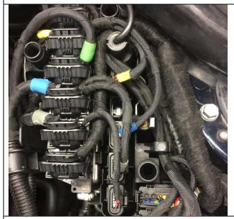
3i.Rout the repaired harness as shown and connect A368\*1B.
