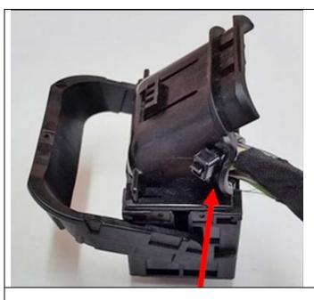
3b. Remove the cable strap (arrow) on both connector A368\*1B and the repair harness.
