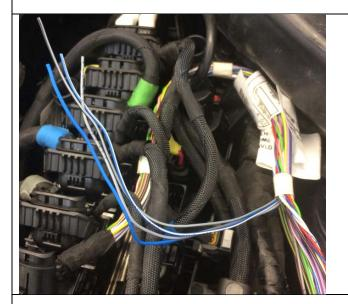
3d. Route the repair harness in the installation position (Repair Kit 61 12 8 793 506).
