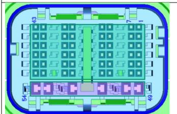
2e. Install suitable sealing plugs (Repair kit P/N 61 12 8 794 765) into all of the open chambers.
