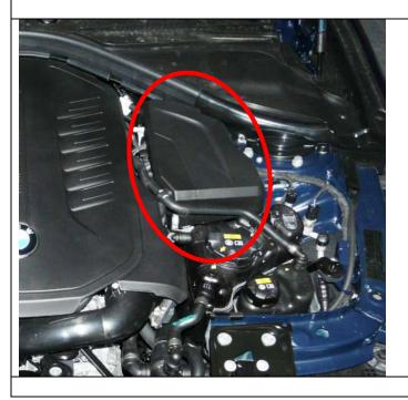
1b. Remove the cover of the DME control unit (circled, shown on B58 engine).
