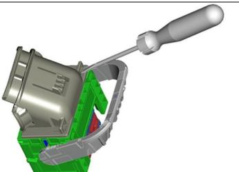
2b. Carefully remove the protective cap from the connector using a suitable tool.
