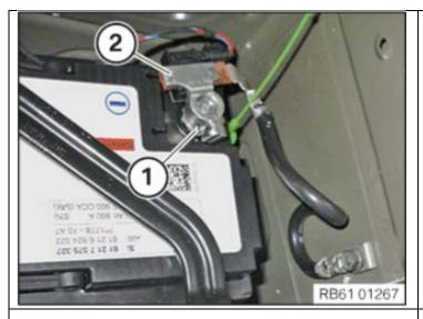
3k.Connect battery earth lead with intelligent battery sensor (IBS) (2) to negative battery terminal.
