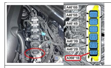
1c. Locate connector A368\*1B and remove it from the DME.
