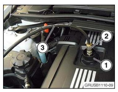
Remove the engine oil cap and install the special pressure tester adapter, P/N 83 30 0 496 326 (1). Connect the quick disconnect coupler (2) onto the pressure tester adaptor. Connect the IMIB pressure measurement hose, P/N A5E0134072 (3).
