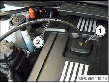
Remove the engine oil cap and install the oil cap adapter (1). Connect the IMIB pressure measurement hose, P/N A5E0134072 (2).
