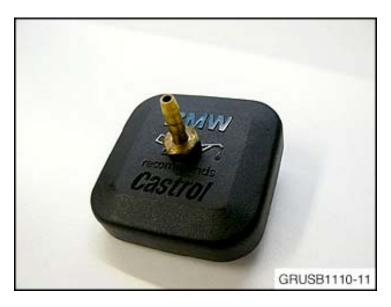
Remove the oil cap adaptor from the existing Slack Tube Manometer.
