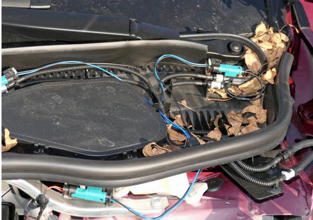
iX: Check the windshield cowl area. Clear any debris from the driver and passenger side water drains.
