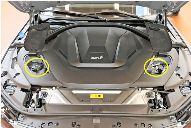
i4: Coolant system reservoir and climate valves (circled) are located under access flaps.
