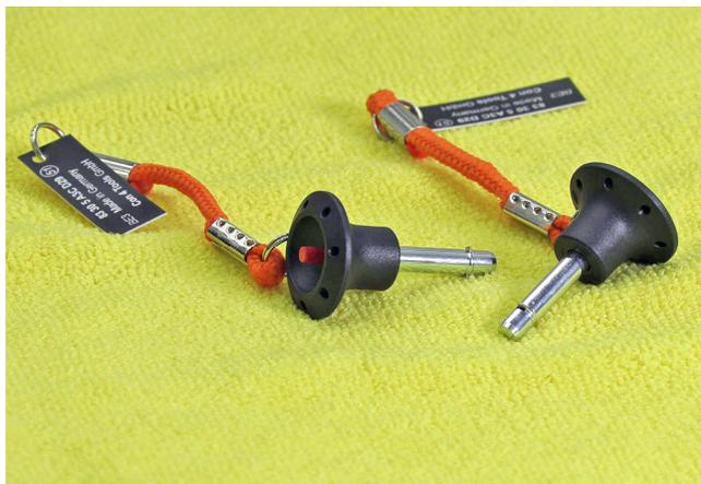
Use special tool P/N 83 30 5A3CD29 to hold the hood open when the tools are inserted into the left and right hood hinges.
