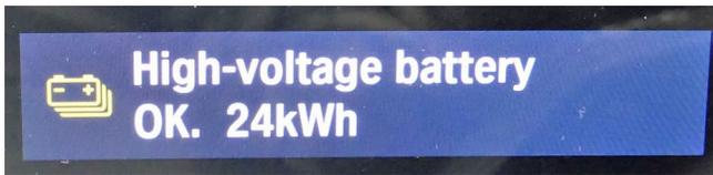
The CID shows the relative SoC of the HV battery.
