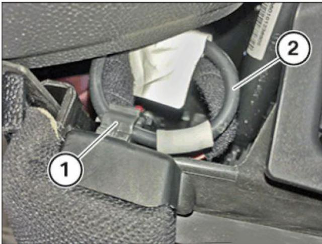
Retaining clip (1) and release loop (2).
