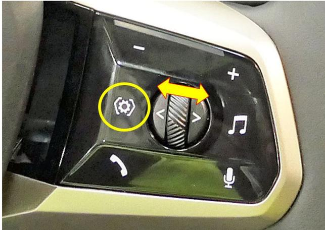
Select different instrument cluster and head-up display layouts by pressing the “Settings” switch (circled).
