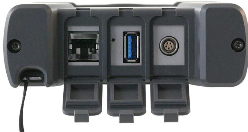
Fig. 2: Interfaces on the ICOM NEXT A, from left to right: RJ45, reset button, USB 3.0 port, jack
