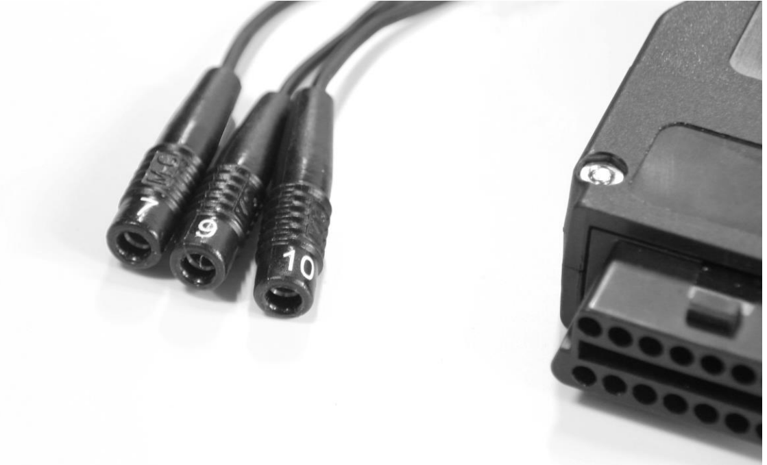
Fig. 13: Measuring sockets with clearly labelled pin indices
