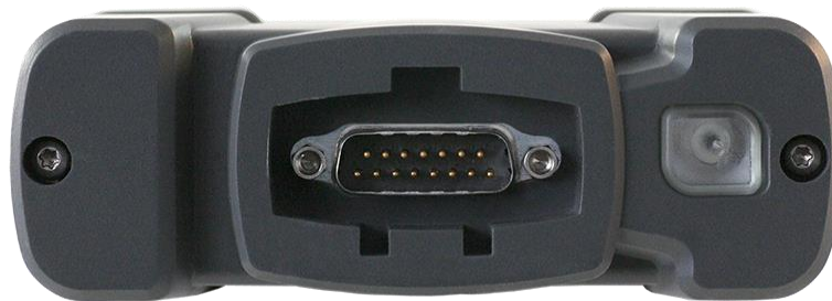
Fig. 1: Sub D socket on the ICOM NEXT A with guide slots for securing the connecting cable (right side: illuminated button for workshop interaction)
