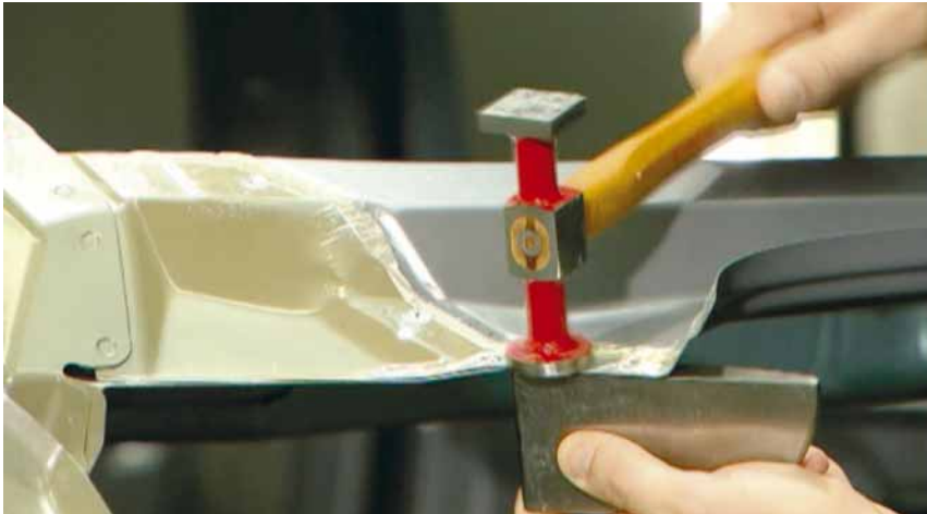
Damaged sheet metal flange
