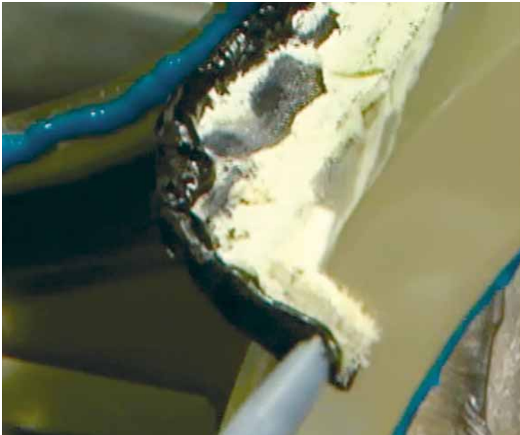
Adhesive on cavity sealing
